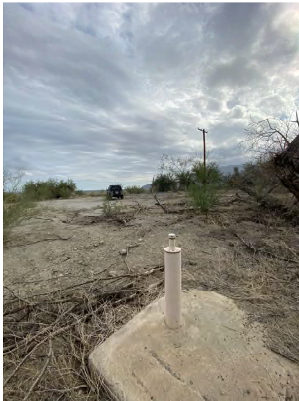
Subject Property; presumed agricultural monitoring well associated with W3.
