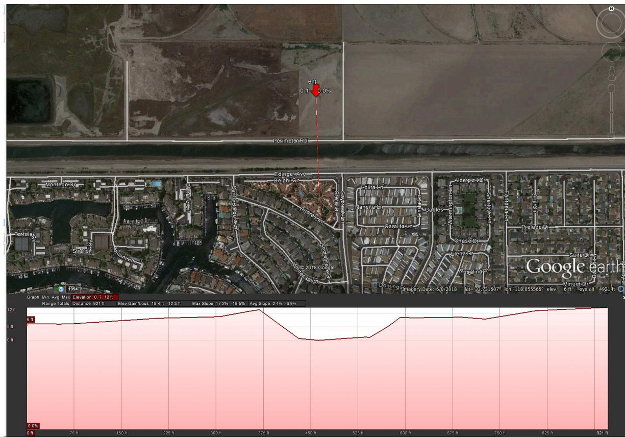
Figure 24b. Impact area C02_1, section – Google Earth (checking bottom ditch elevation)
