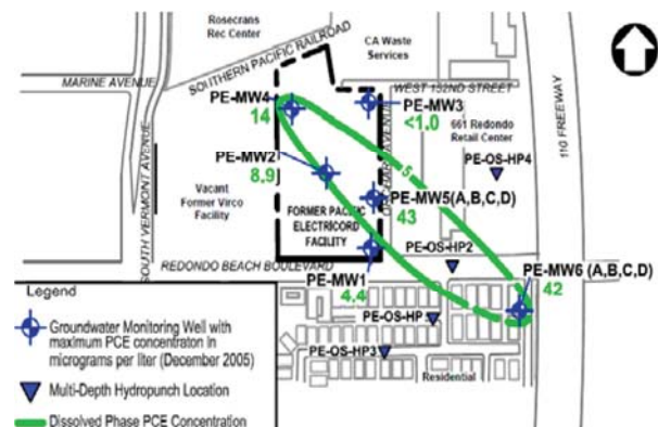
Figure 1: Site Location Map showing PCE concentrations in groundwater
