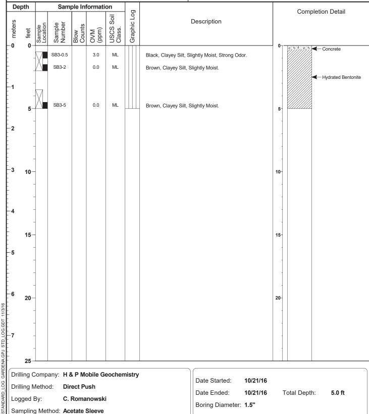
Drilling Company: H & P Mobile Geochemistry
