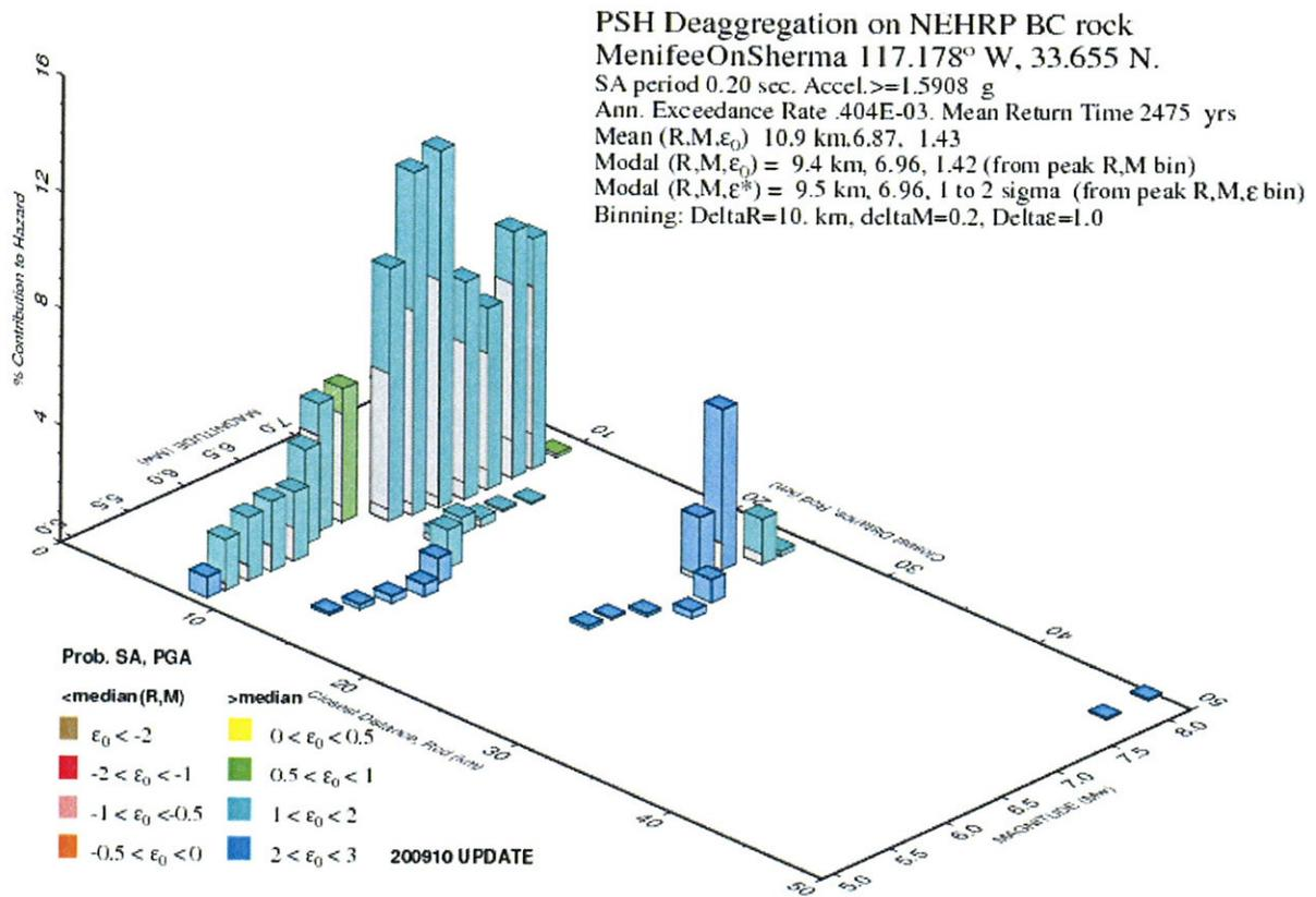
GMT 2016\_Jan 1 00:05:27 Distance (R), magnitude (M), epsilon (E,E) deaggregation for a site on rock with average vs=760. m/s top 30m. USGS CGHT PSHA2008 UPDATE Bins with 110.09% contrib. omitted
