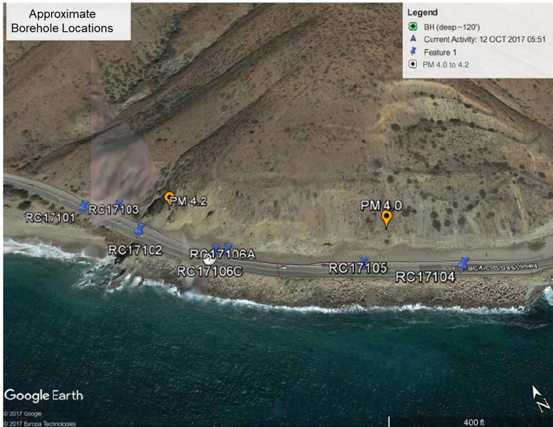
**Figure 2-10: Approximate borehole locations for geotechnical borings. The shallow boring RC17106B is not mapped but is located at very close proximity to RC17106A.**
