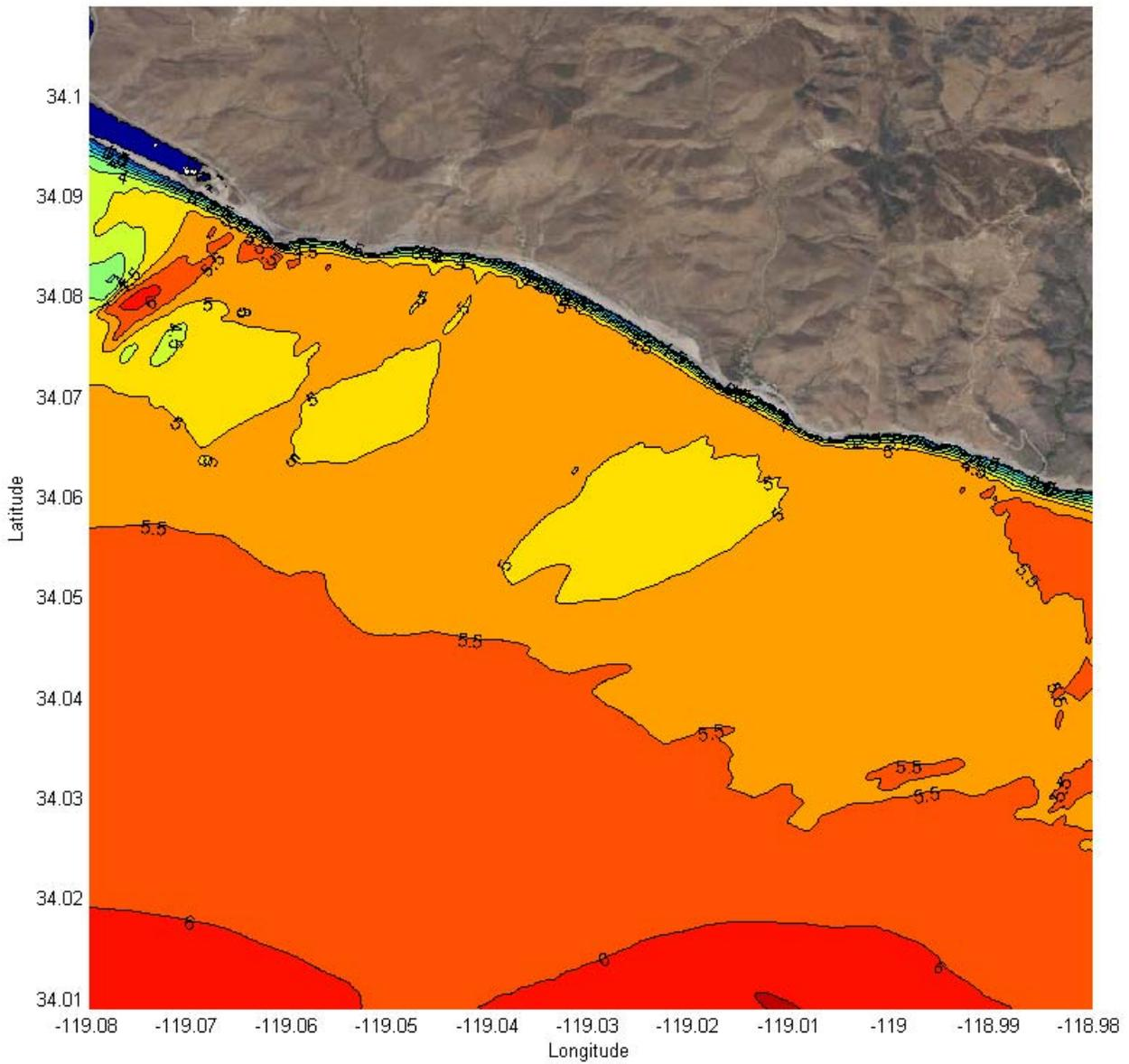
**Figure 27: SWAN model results on the fine grid showing contours of Hs (m) with initial conditions of 100 year wave height (21.7 feet), wave direction of 240 deg. and a peak wave period 16 sec.**
