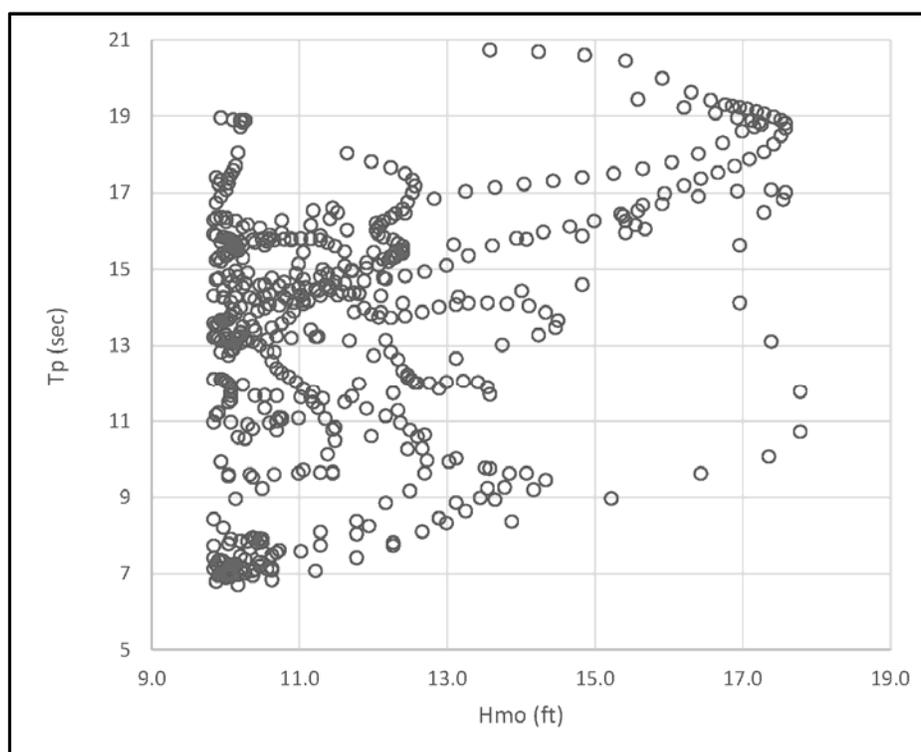
**Figure 23:** Scatter plot of wave height vs. wave period for all waves in excess of 10 feet at WIS Station 83096.
