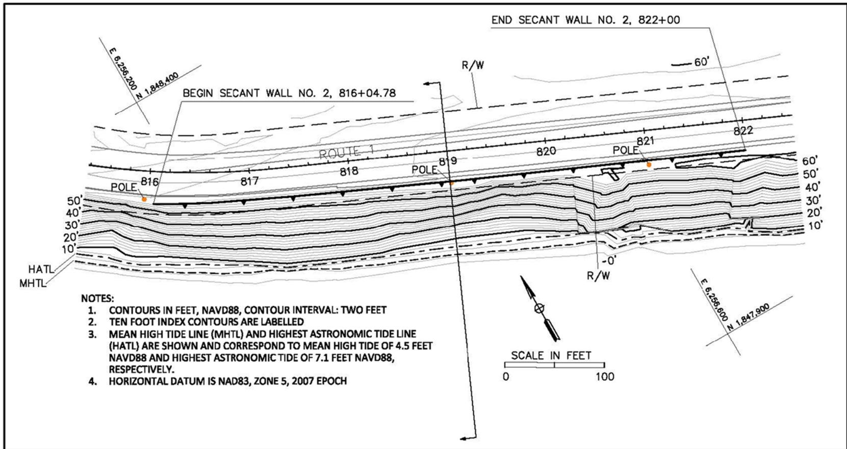
Figure 3-6: Plan view of the proposed secant wall and surrounding topography at PM 4.0.
