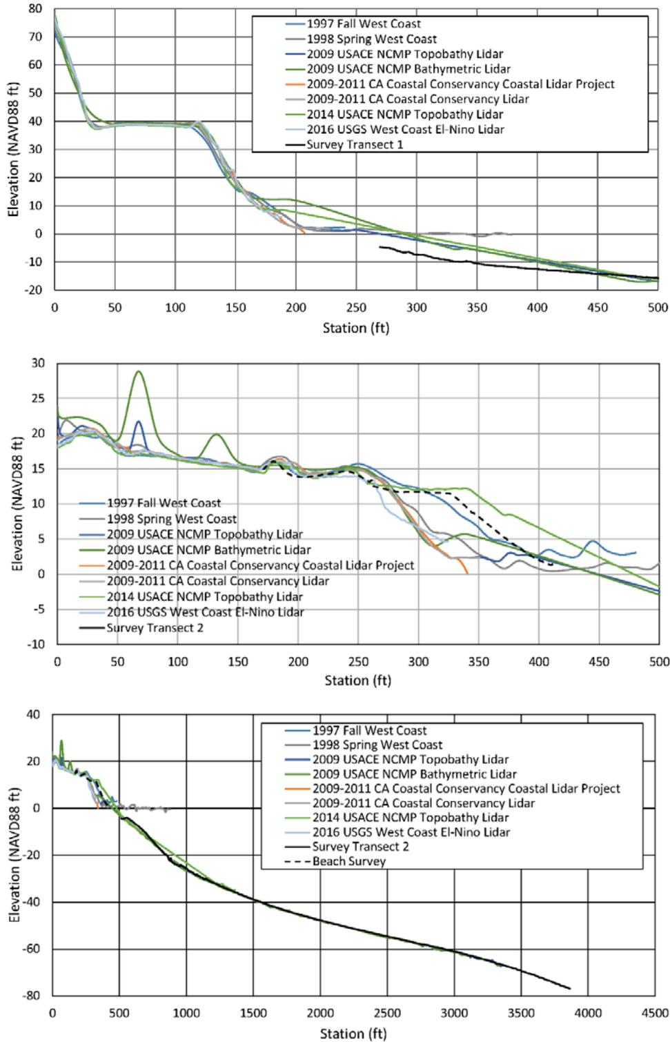
**Figure 17: Shoreline profiles based on lidar surveys and the surveys for this study. Top and middle show transects T-1 and T-2, respectively. The bottom shows the whole transect for T-2.**
