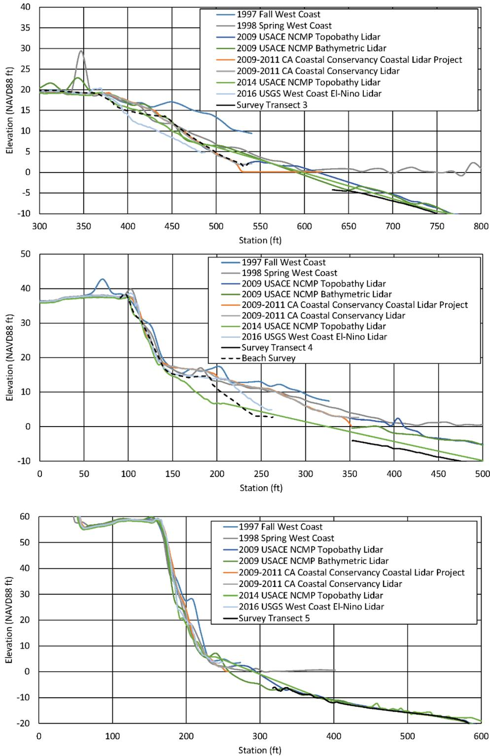
**Figure 18: Shoreline profiles based on lidar surveys and the surveys for this study. Top to bottom show transects T-3, T-4 and T-5.**
