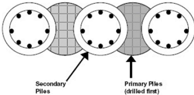
**Figure 1-18: Typical Schematic Plan View of a Secant Pile Wall**
