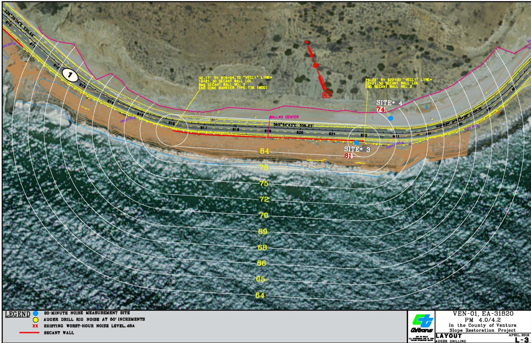
Figure 2-15: Construction noise contour lines with the peak traffic noise values modeled at PM 4.0.
