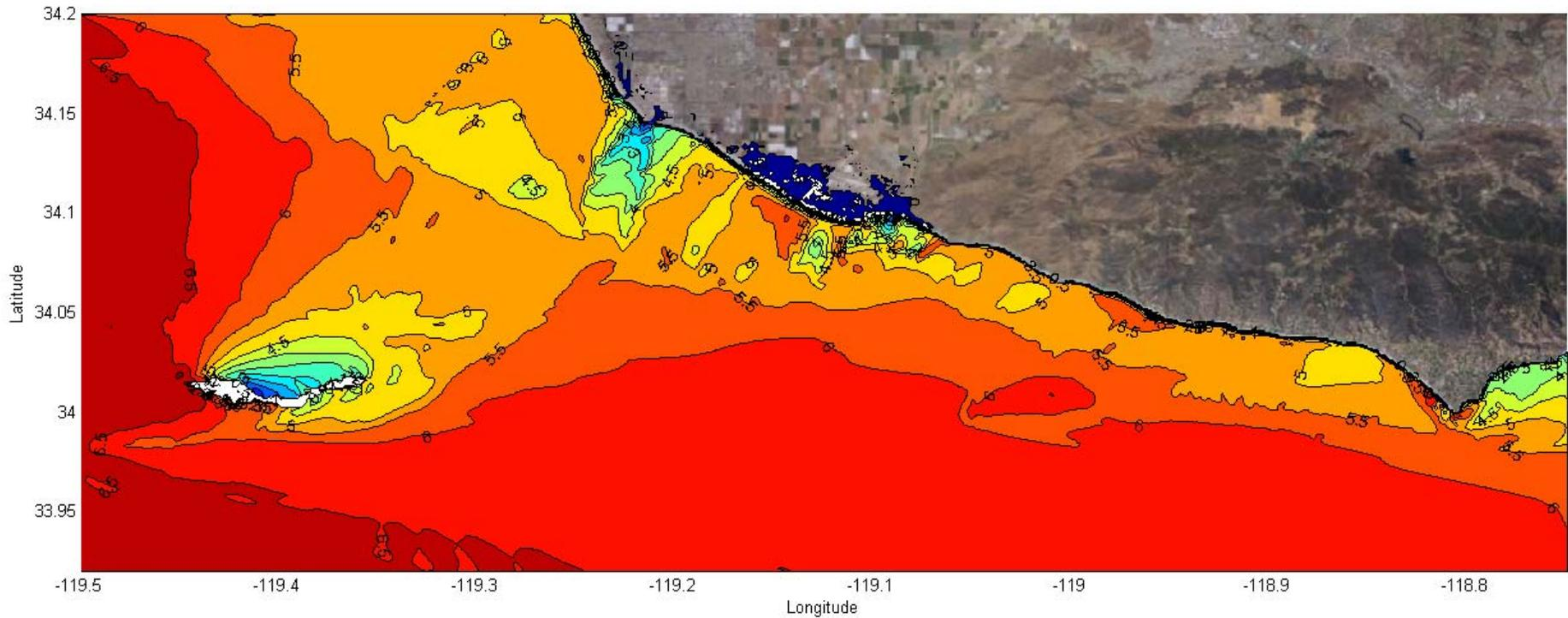
Figure 26: SWAN model results on the south coarse grid showing contours of  $H_s$  (m) with initial conditions of 100 year wave height (21.7 feet), wave direction of 240 deg. and a peak wave period 16 sec.
