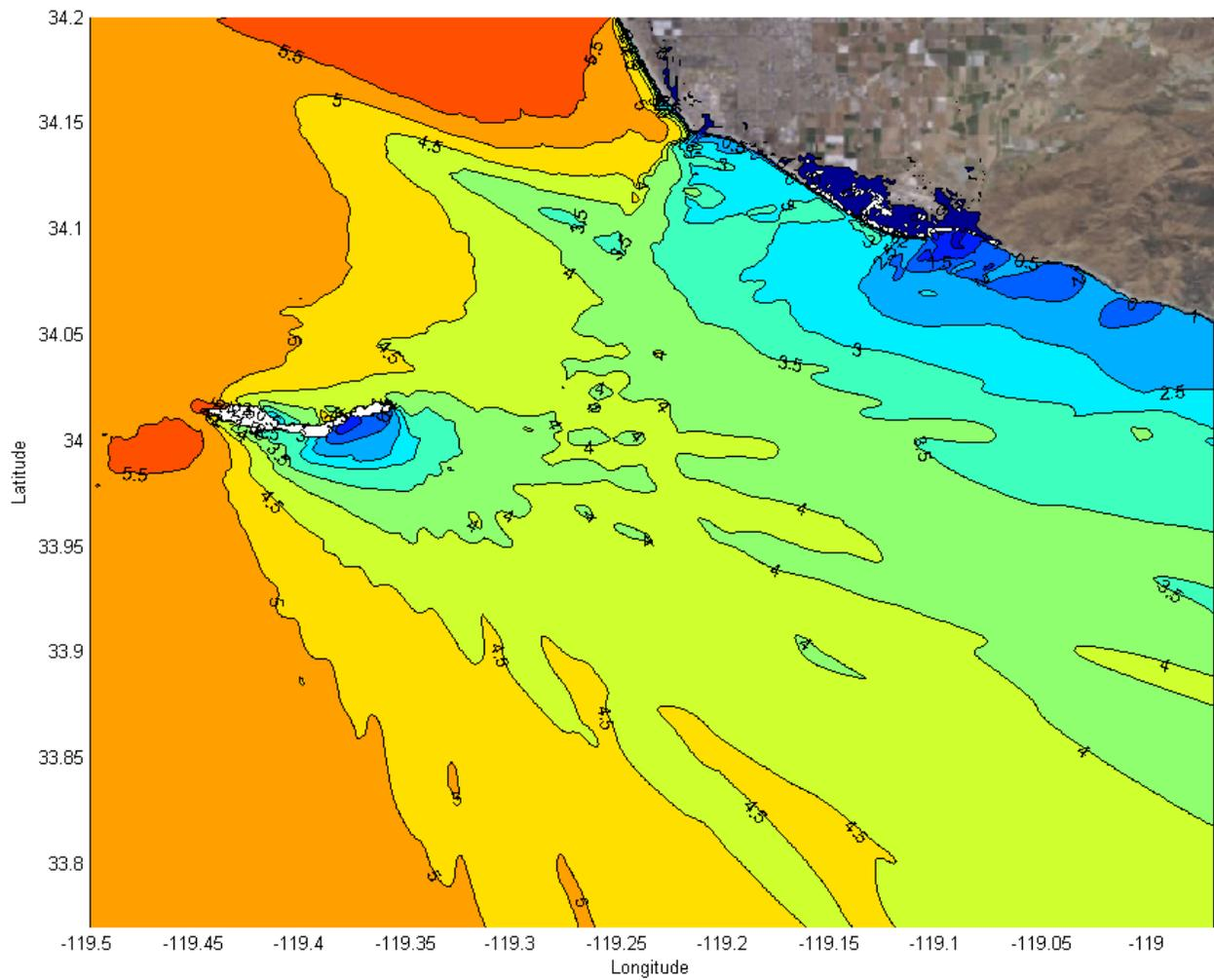
**Figure 28: SWAN model results on the west coarse grid showing contours of Hs (m) with initial conditions of 100 year wave height (17.7 feet), wave direction of 330 deg. and a peak wave period 16 sec.**
