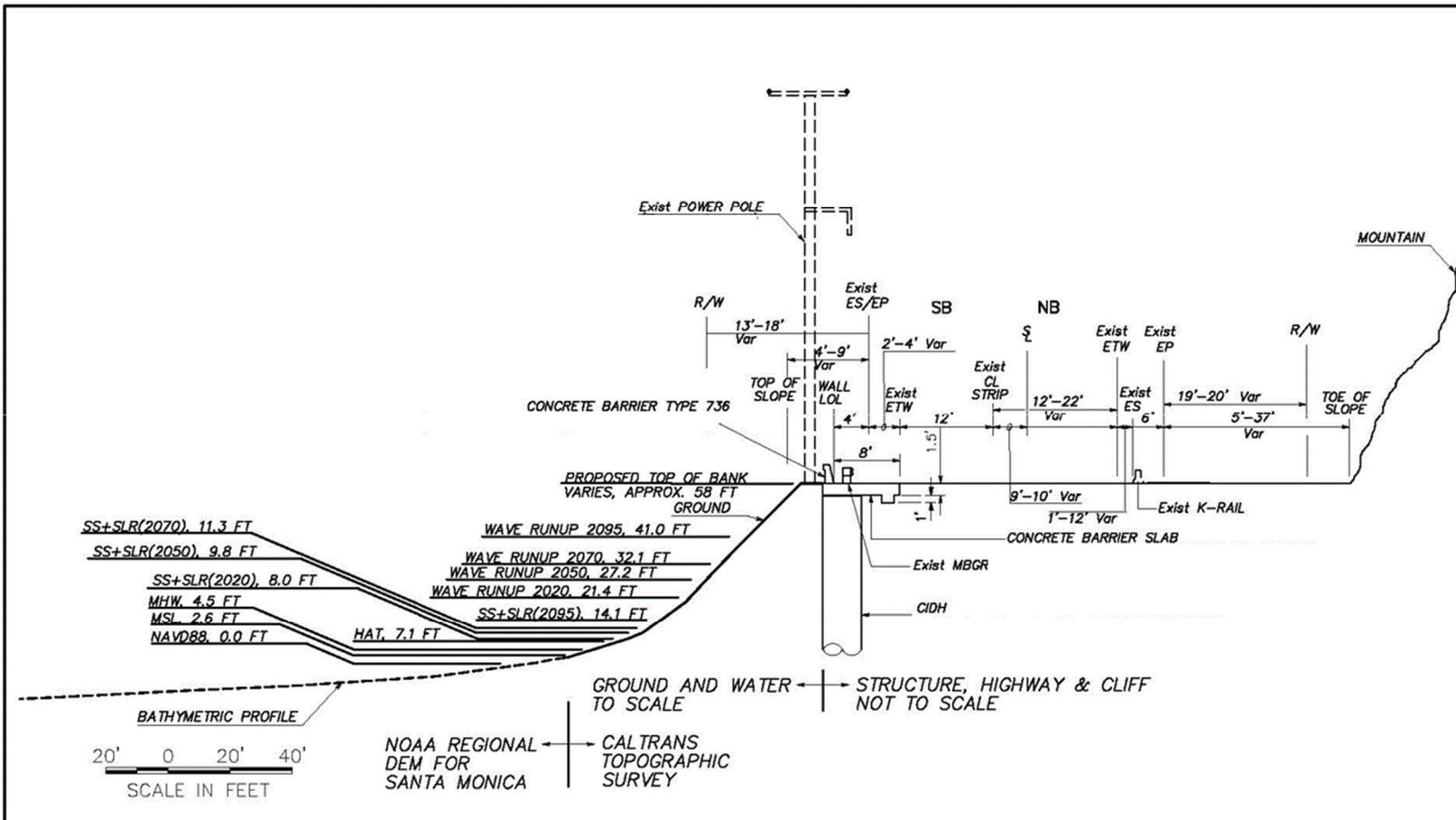
Figure 3-8: Cross section view of the proposed secant wall and applicable water levels at PM 4.0
