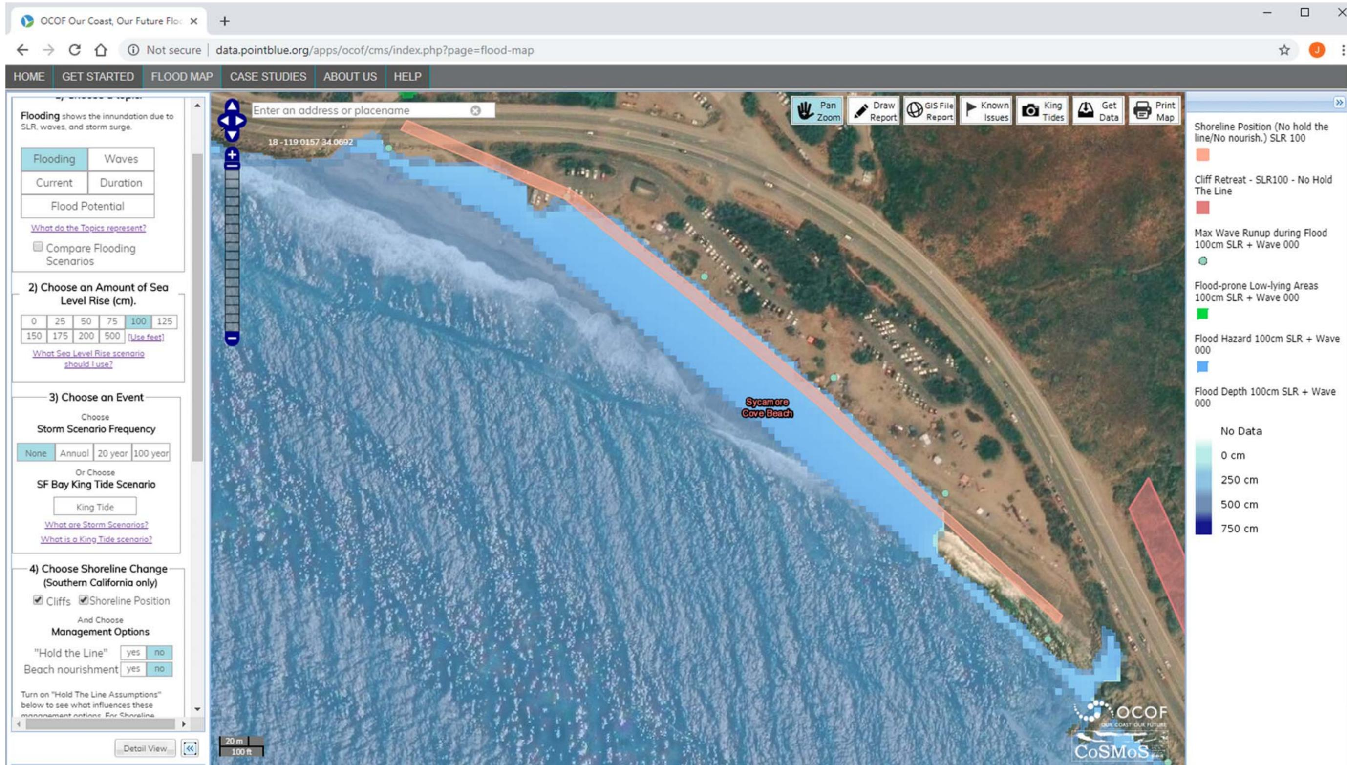
Figure A-5-3: CoSMoS schematic showing shoreline for sea level rise of 3.3 feet (100 cm), approximating year 2070 for this study.
