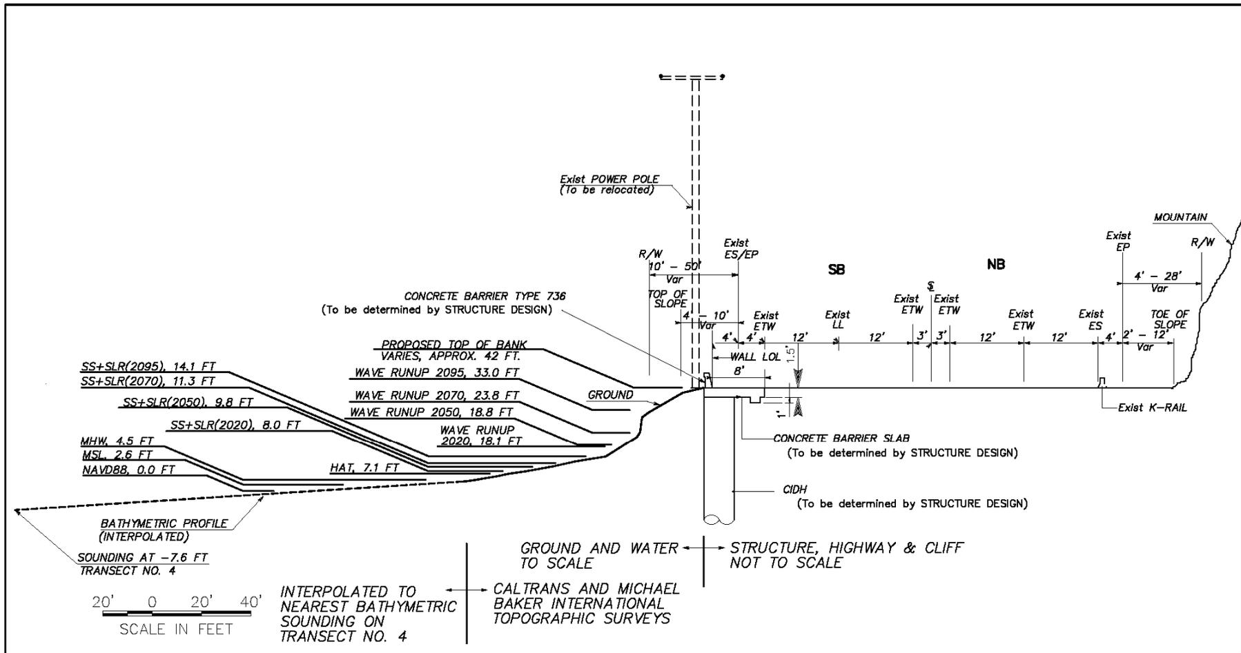
**Figure 38: Cross section view of the proposed secant wall and applicable water levels at transect T-4 (PM 4.2).**
