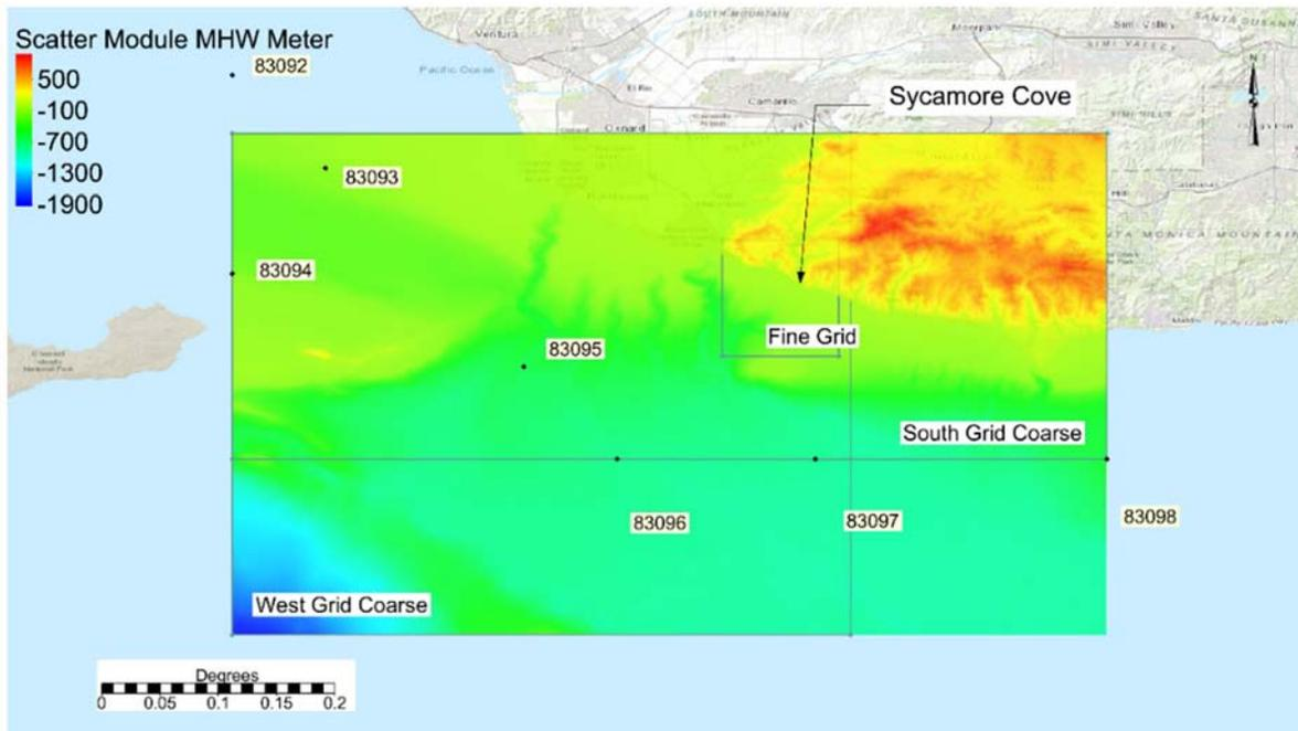
**Figure 25: The coarse and fine grids along with the bathymetry and WIS stations.**
