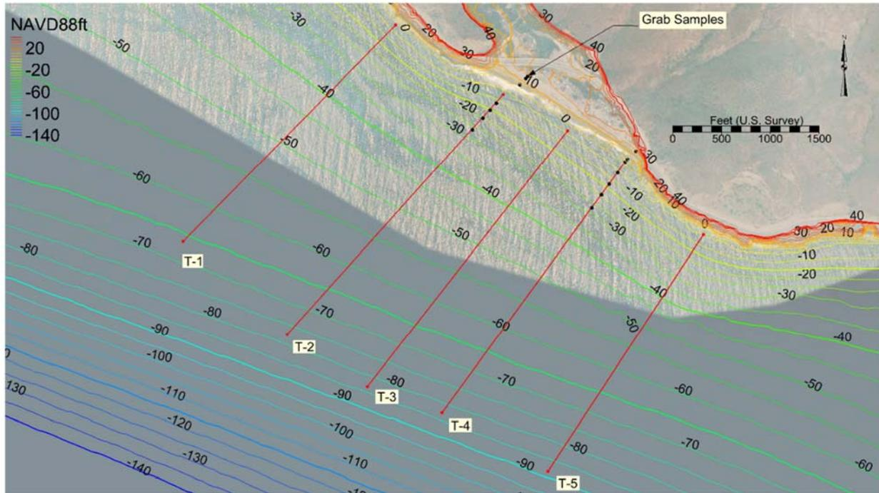
**Figure 8: Bathymetric contours close to the project site/ location of bathymetric transects T-1 through T-5.**
