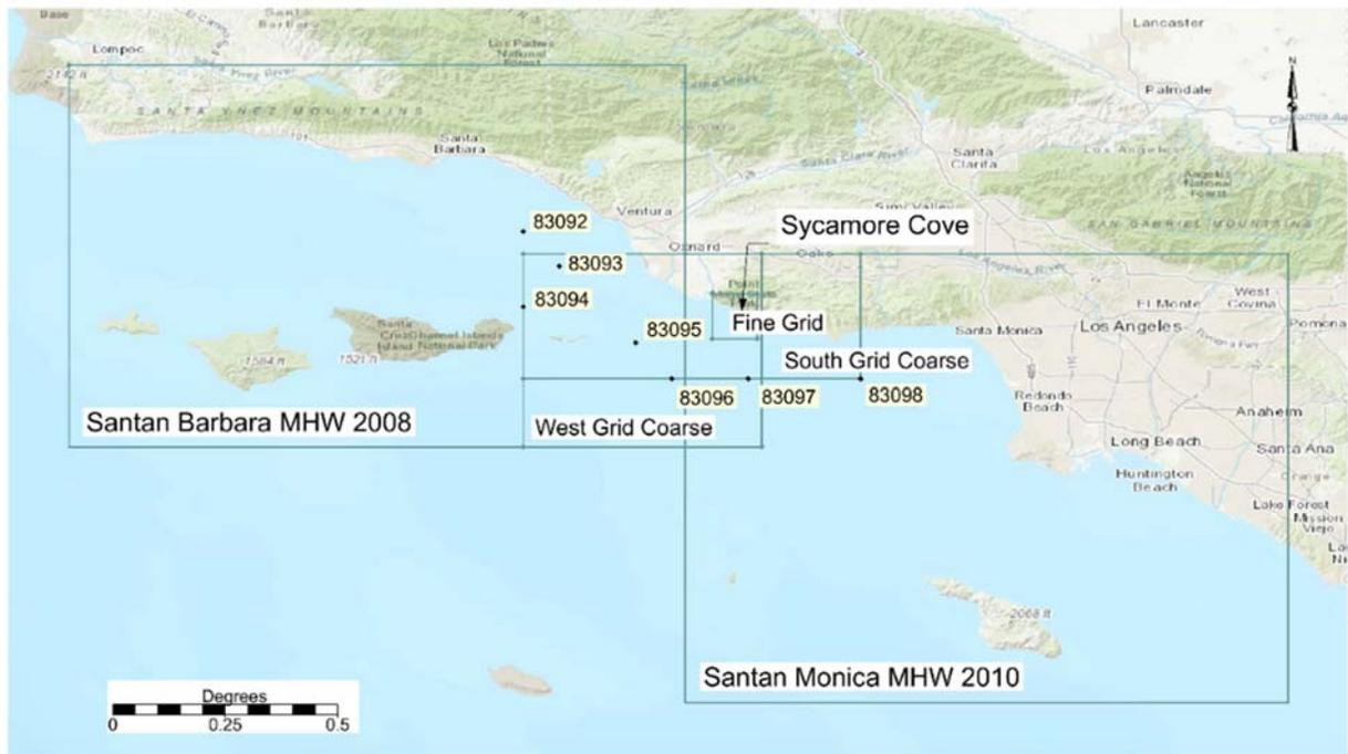
**Figure 24: Regional digital elevation models used to develop the two coarse grids and the fine grid used in the SWAN model.**
