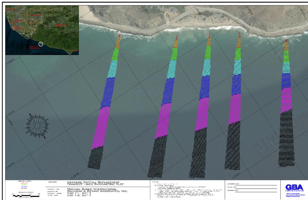
Figure 7: Multibeam hydrographic survey along five transects, Oct. 11-13, 2017.
