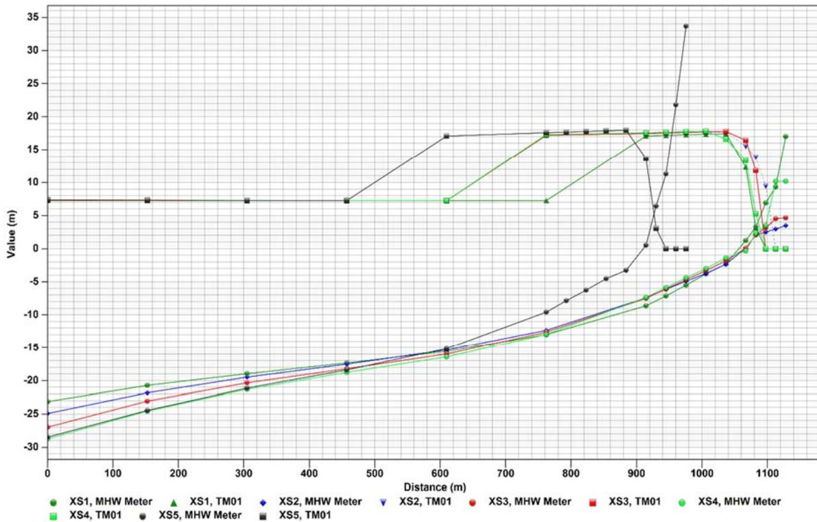
Figure 31: Plot of the peak wave period  $T_p$  associated with the wave height shown in Figure 30 and depth relative to MHW (i.e. SWAN model datum) for 100 year wave and 2100 high water level scenario.
