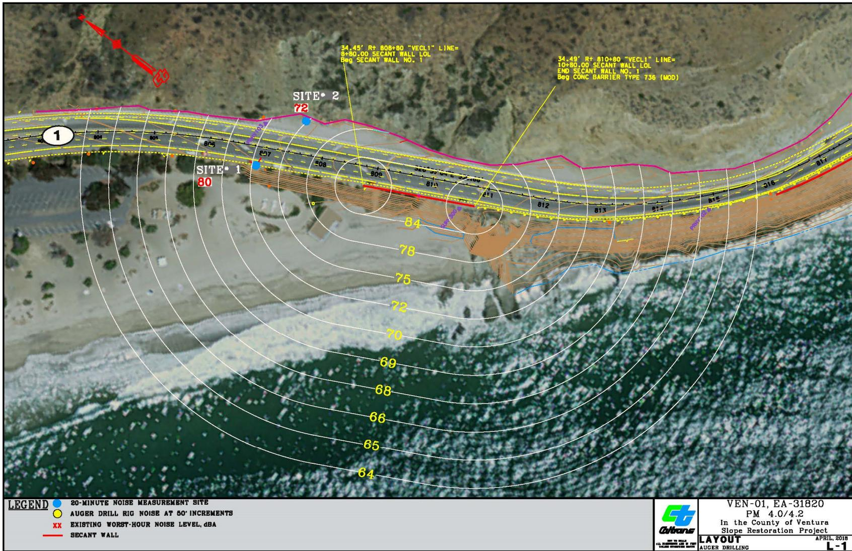
Figure 2-14: Construction noise contour lines with the peak traffic noise values modeled at PM 4.2.
