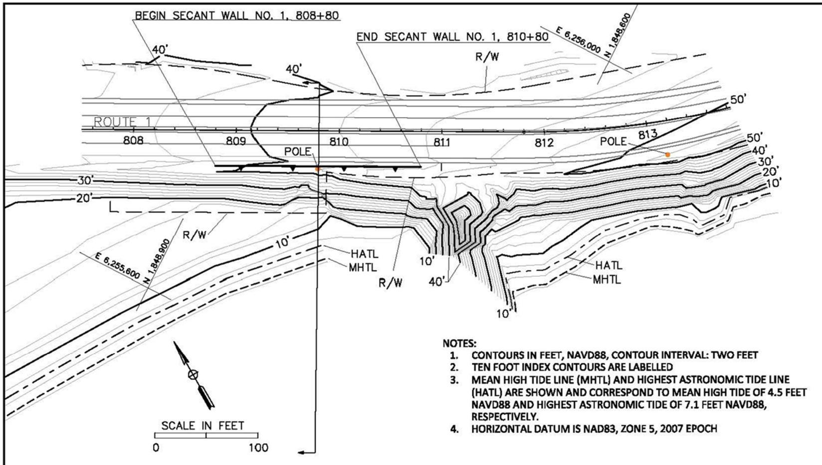
Figure 3-7: Plan view of the proposed secant wall and surrounding topography at PM 4.2.
