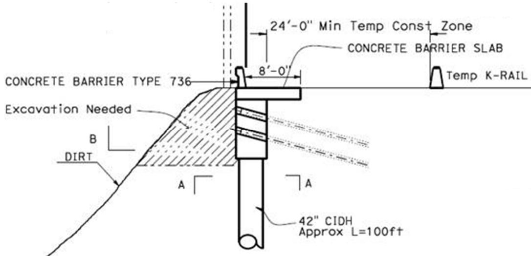
**Figure 1-21: Schematic drawing of Alternative 2 – Ground Anchor Option.**
