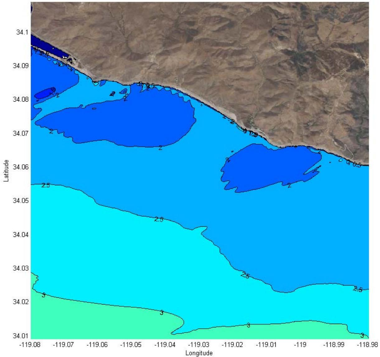
**Figure 29: SWAN model results on the fine grid showing contours of Hs (m) with initial conditions of 100 year wave height (17.7 feet), wave direction of 330 deg. and a peak wave period 16 sec.**
