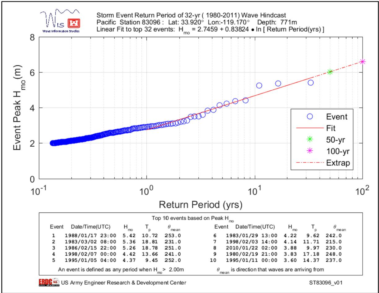
**Figure 21: Probability of a given deep water offshore wave height in a given year.**
