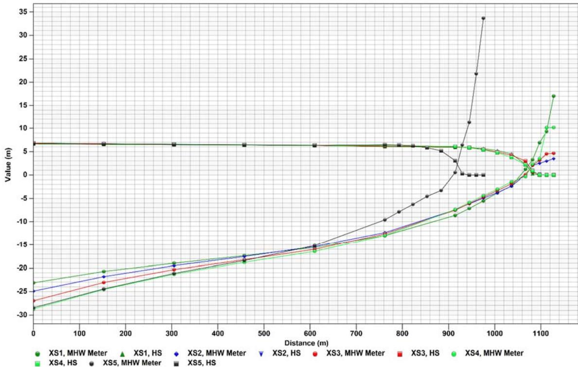
**Figure 30: Plot of the significant wave height Hs and depth relative to MHW (i.e. SWAN model datum) for 100 year wave and 2100 high water level scenario.**
