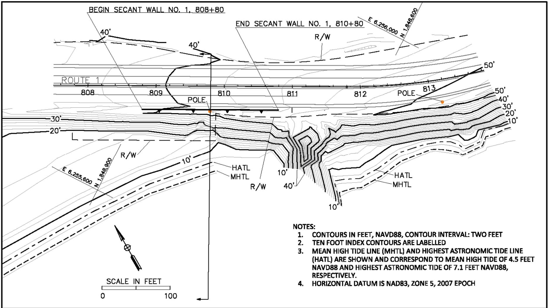
**Figure 37:** Plan view of the proposed secant wall and surrounding topography at transect T-4 (PM 4.2).
