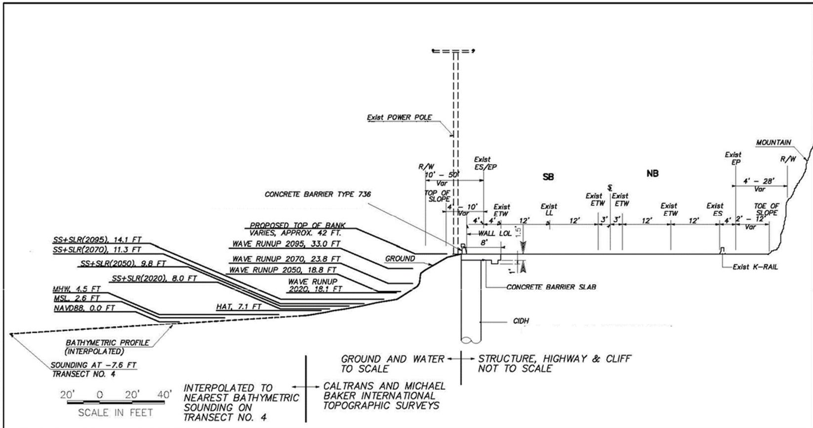
Figure 3-9: Cross section view of the proposed secant wall and applicable water levels at PM 4.2.
