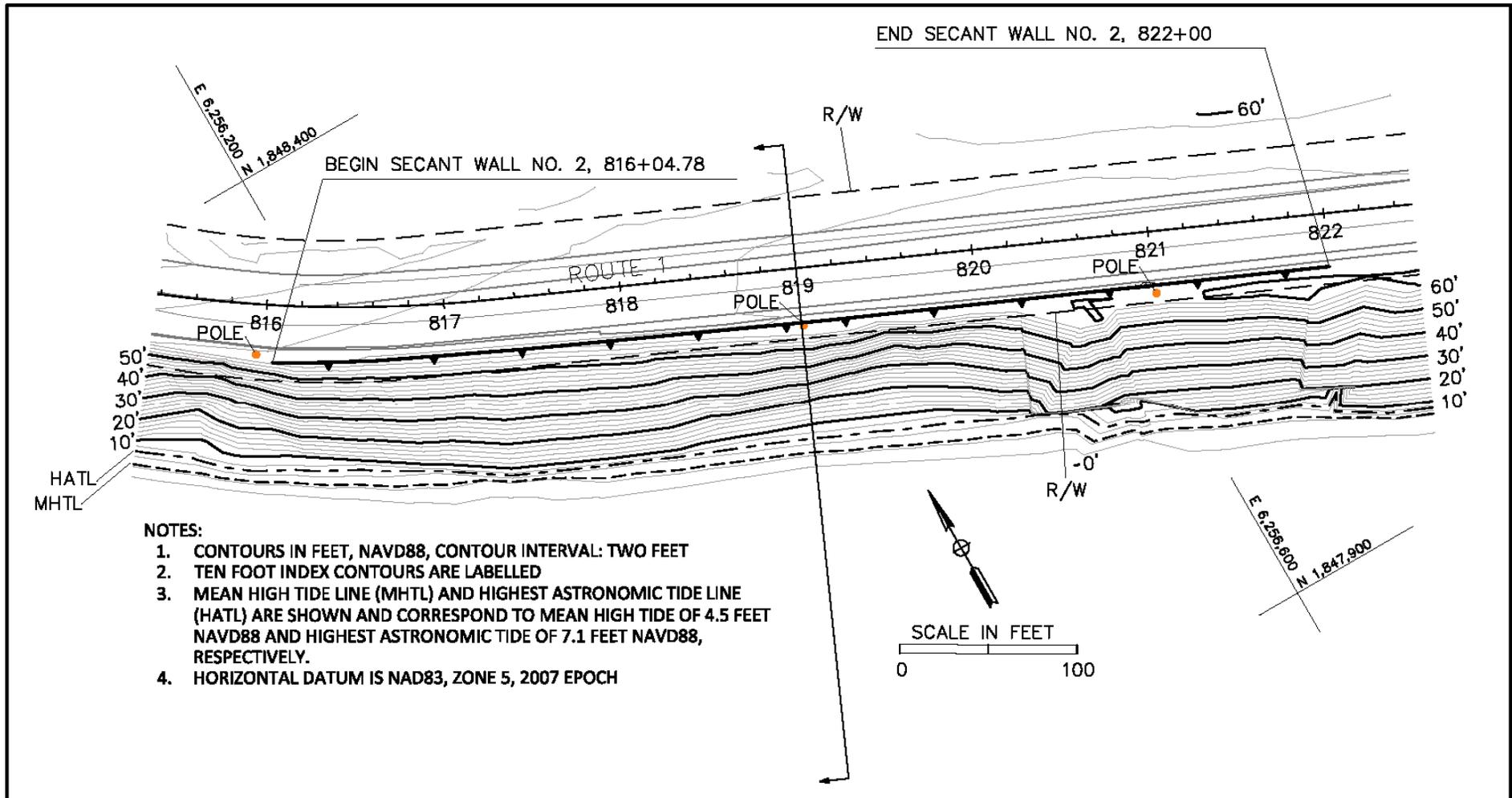
**Figure 35:** Plan view of the proposed secant wall and surrounding topography at transect T-5 (PM 4.0).
