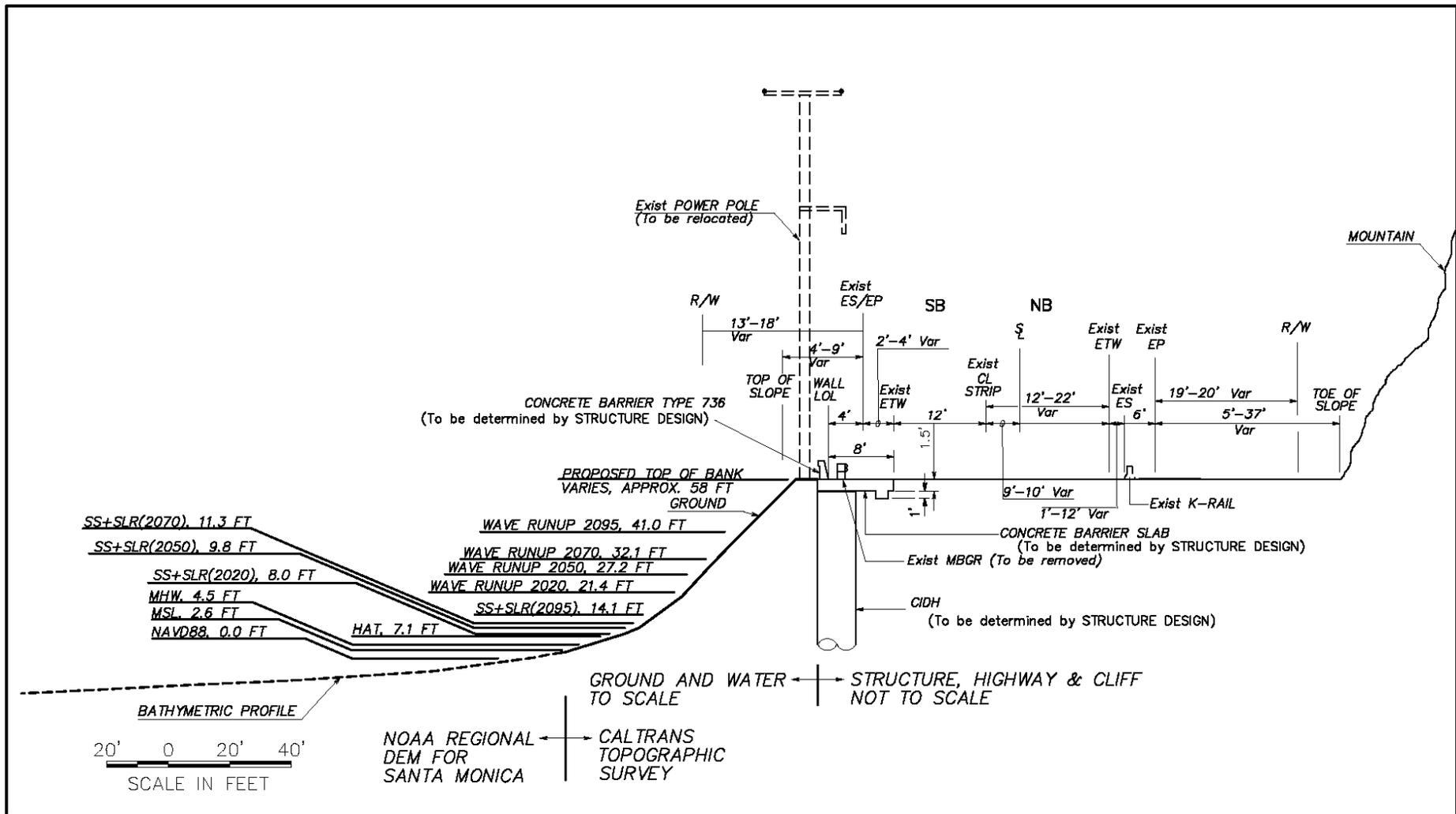
**Figure 36: Cross section view of the proposed secant wall and applicable water levels at transect T-5 (PM 4.0).**
