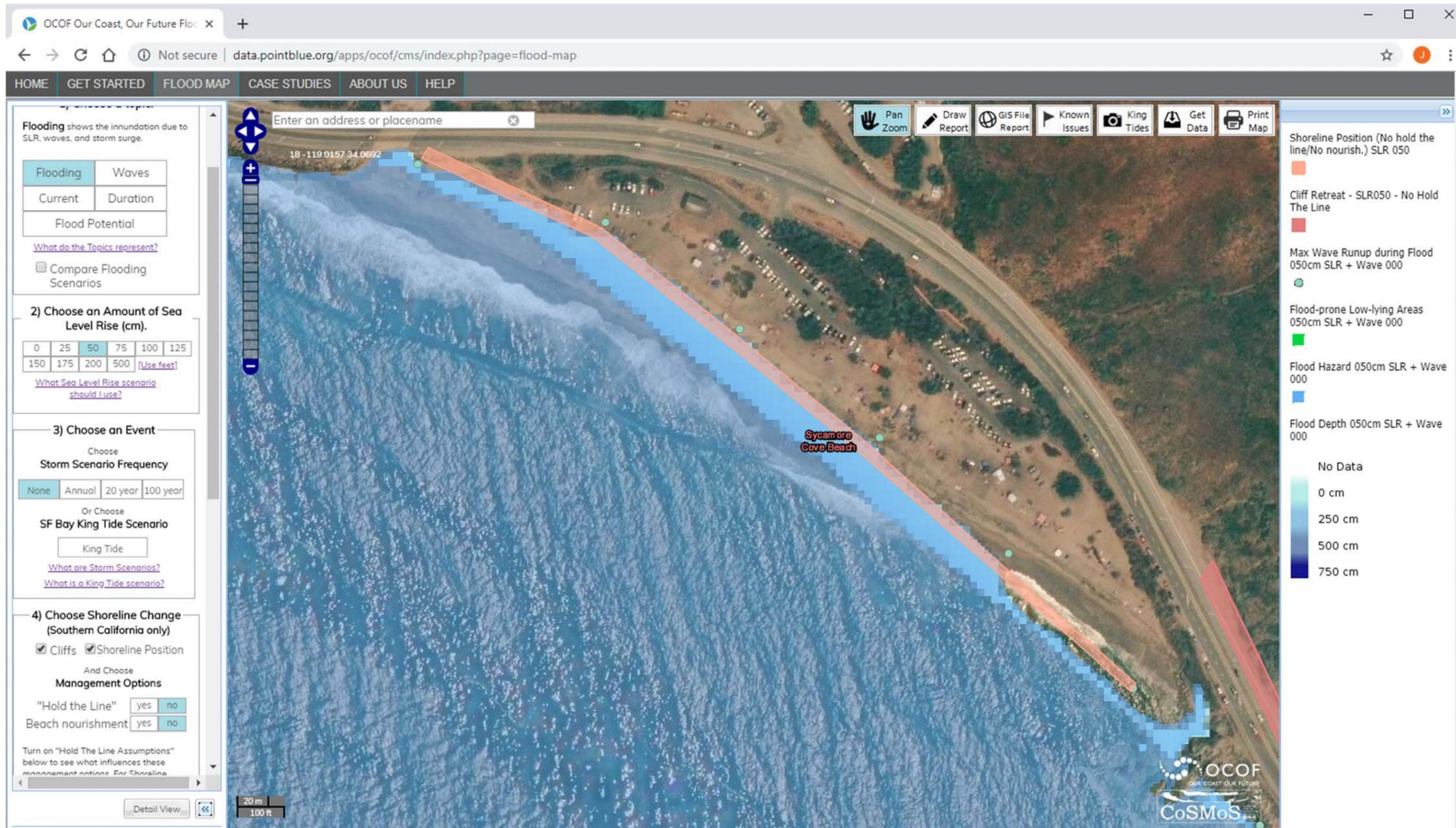
Figure A-5-2: CoSMoS schematic showing shoreline for sea level rise of 1.6 feet (50 cm), approximating year 2050 for this study.
