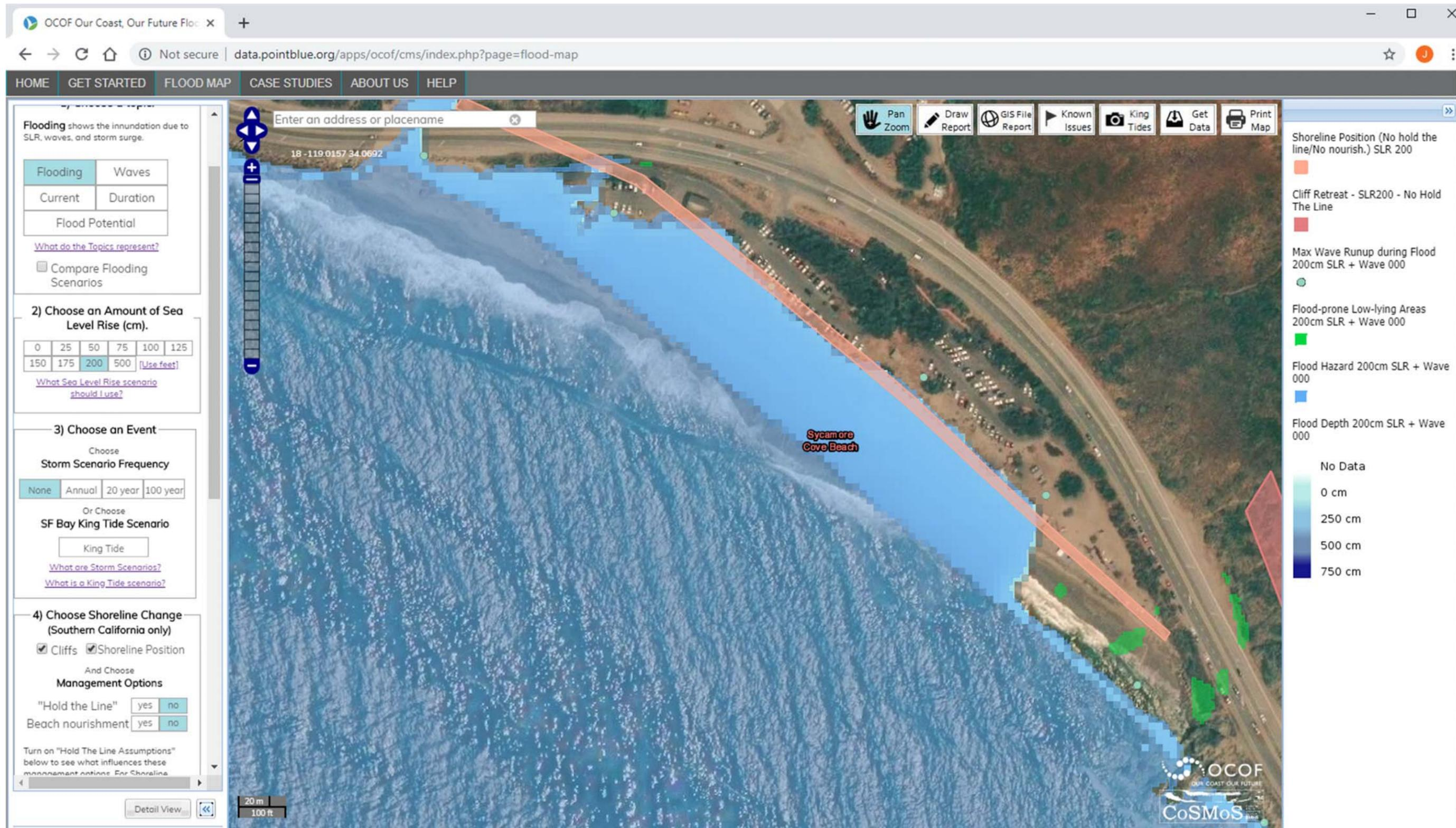
Figure A-5-4: CoSMoS schematic showing shoreline for sea level rise of 6.6 feet (200 cm), approximating year 2095 for this study.
