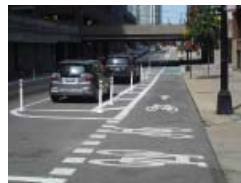
Class IV: Cycletrack Provides a separated right-of-way for the exclusive use of bicyclists adjacent to a roadway
