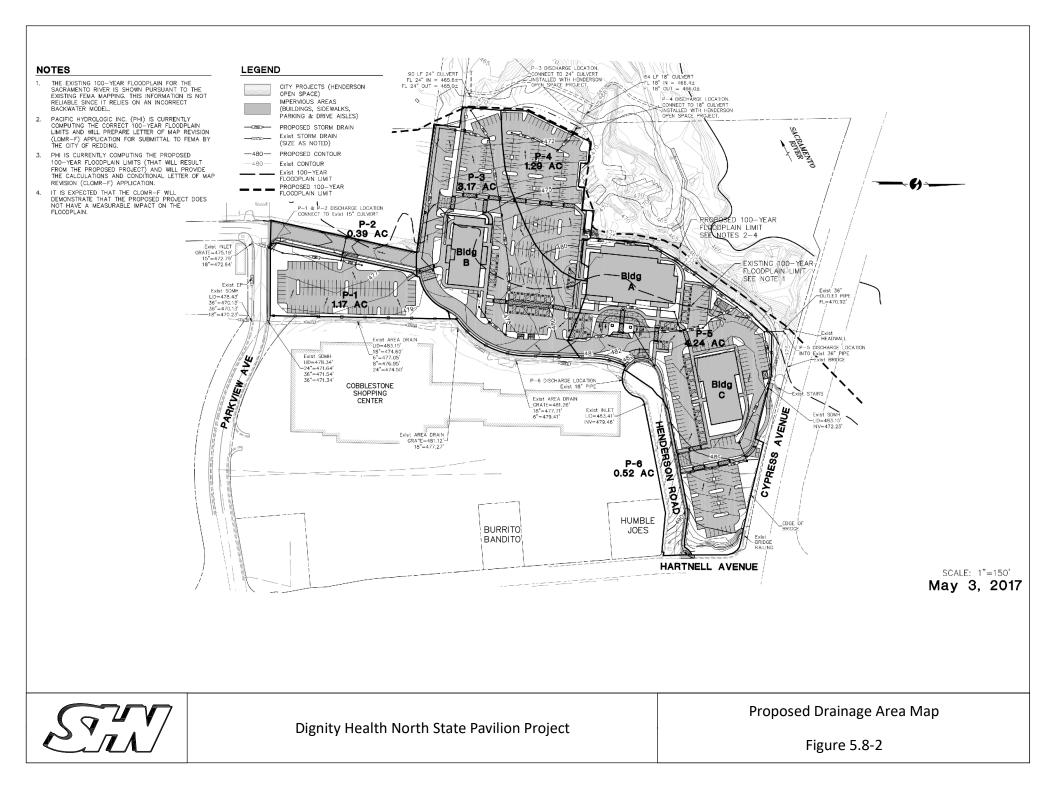
As noted in Table 5.8-4, upon project completion the impervious area would increase from 27 percent to 77 percent. The proposed 10-year, 25-year, and 100-year peak flows for the entire project site are 44 cfs, 51 cfs, and 66 cfs, respectively. This amounts to an increase of 18 cfs, 20 cfs, and 20 cfs for the 10-year, 25-year, and 100-year peak flows, respectively.
