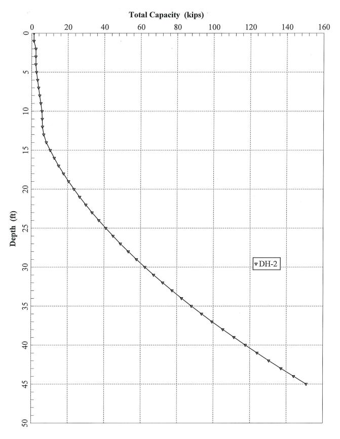
Total Capacity of pile vs. Depth
