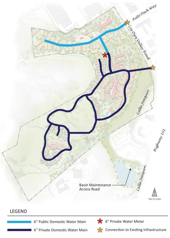
Figure 6-1 Water Supply Plan
