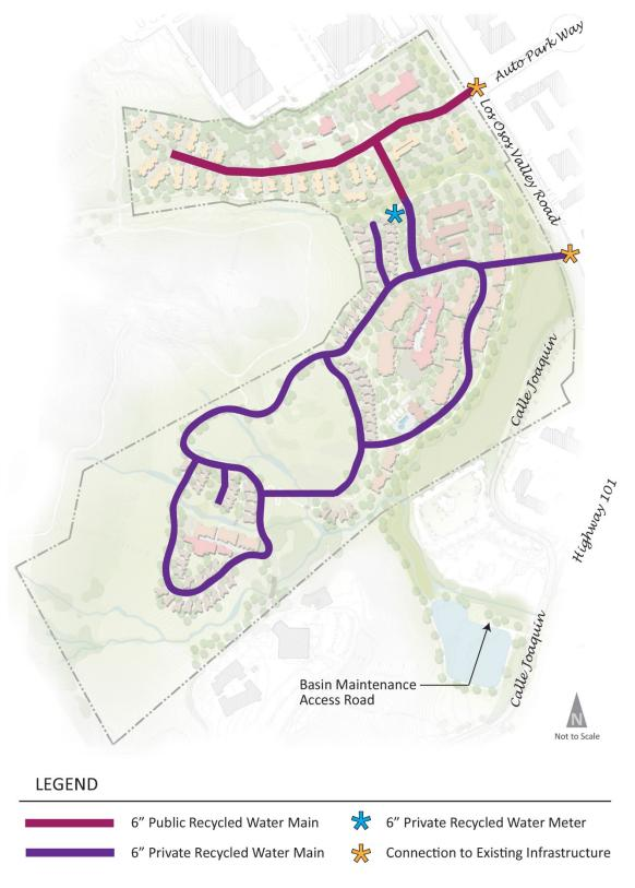
Figure 6-2 Recycled Water Supply Plan
