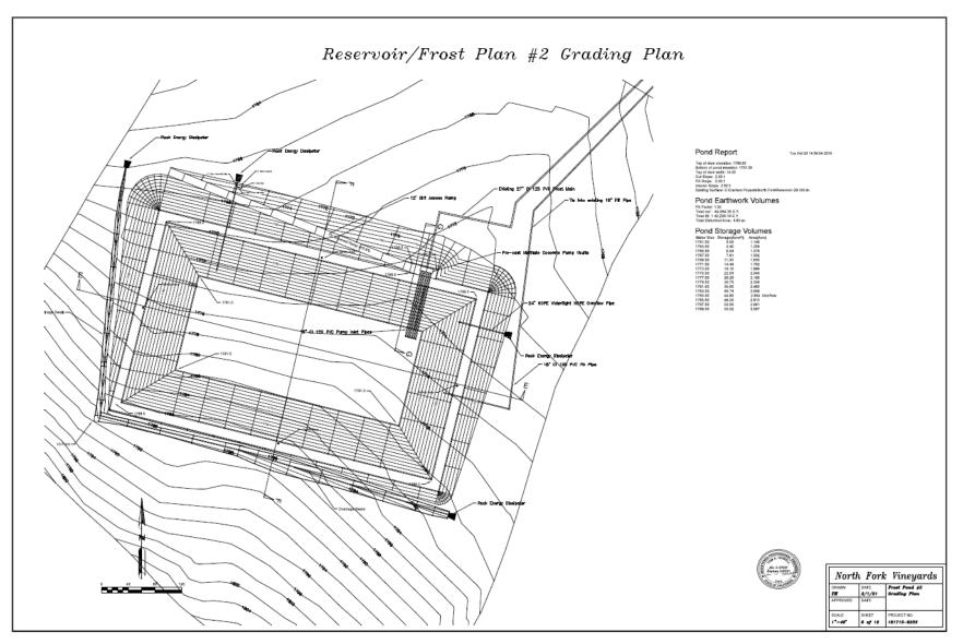
Figure 2-4 Reservoir/Frost Pond #2 Grading Plan
