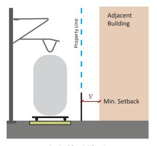
A minimum setback of five (5) feet between an adjacent structure and Metro ROW is strongly encouraged to allow project construction and ongoing maintenance without encroaching on Metro property.
