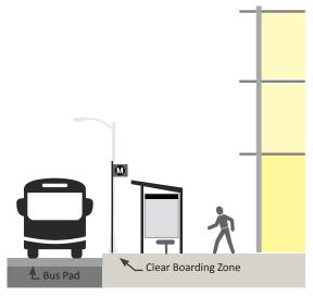
A concrete bus pad should be located at bus stops and bus shelters should be located along sidewalks to ensure an accessible path of travel to a clear boarding area.
