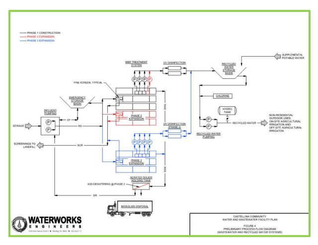
Exhibit 14 - Wastewater Treatment System Schematic
