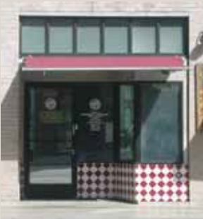
The window sash located above a door. Also called transom light.
