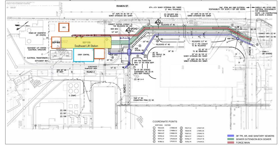
Figure 3: Site Plan for Proposed SEP 005 Lift Station and Associated Pipelines
