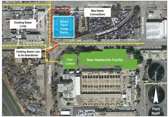
Figure 1: Headworks Replacement Project – Bruce Flynn Pump Station Sewer Connection
