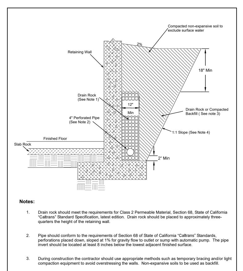
4. Slope excavation back at a 1:1 gradient from the back of footing where expansive materials are exposed.
