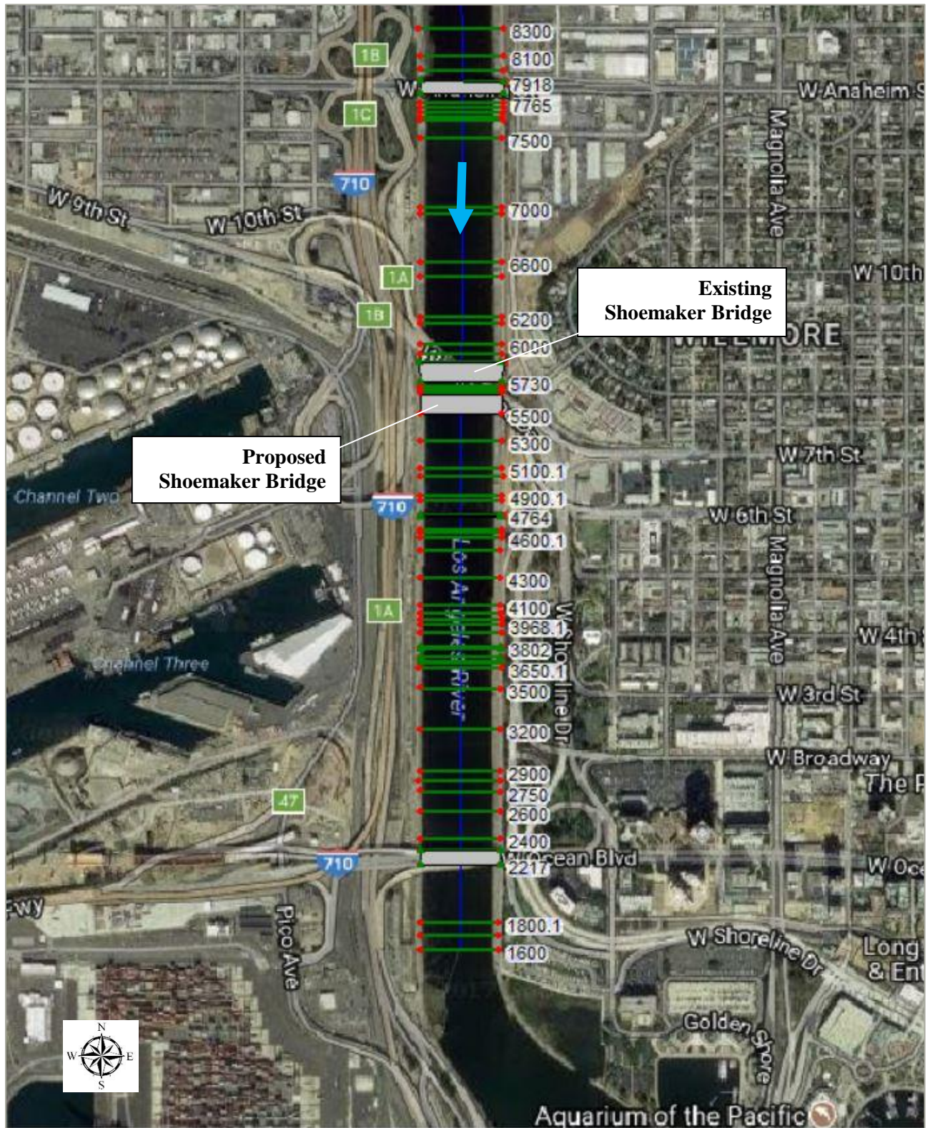
Figure 3-1. Los Angeles River HEC-RAS Model Schematic
