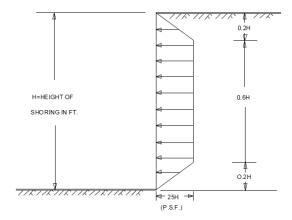
The recommended earth pressure provided above is a preliminary value. The final earth pressure for design of soldier piles and anchors will be provided in the during the design-level geotechnical investigation. Surcharge loads from equipment or stockpiled material should be kept behind the top of the temporary excavations a horizontal distance of at least twice the depth of the excavation.
