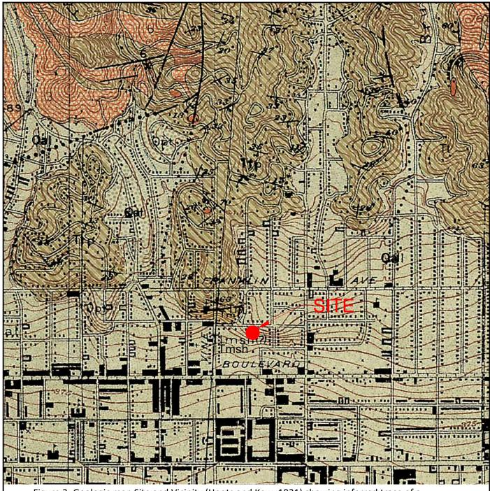
Figure 3: Geologic map Site and Vicinity (Hoots and Kew, 1931) showing inferred trace of a Hollywood Fault separating Modelo ( $T_m / T_{msh}$ ), and Topanga ( $T_t$ ) Formations, granite rocks (gr), and alluvium ( $Q_{al}$ ).
