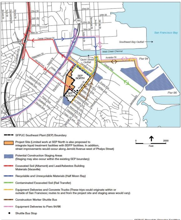
SOURCE: San Francisco Public Works 2005 GIS data; Adavant Consulting and LCW Consulting, Data developed in 2016 for BDFP SFPUC Biosolids Digester Facilities Figure 2-15 Construction Haul Routes
