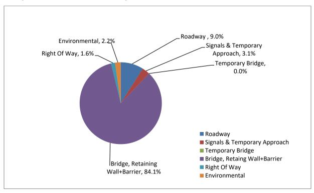
Figure 4-3. CIP Box Girder (Two-Stage) Cost Breakdown
