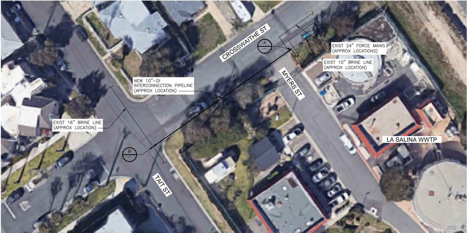
10" CONNECTION TO 16" AT LA SALINA WWTP PLAN 1" = 20'
