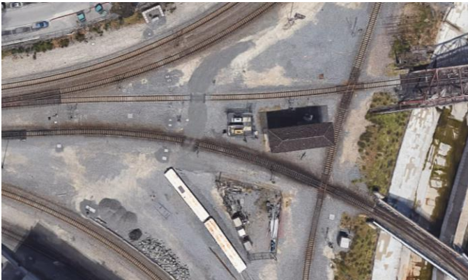
Sunset Line tracks north of Mission Tower, west of Mission Junction Bridge. Satellite imagery dated 2018, courtesy of Google Maps. Note section of missing ties at left. (Track locations within the study area were unsafe and/or inaccessible for project team to photograph.)
