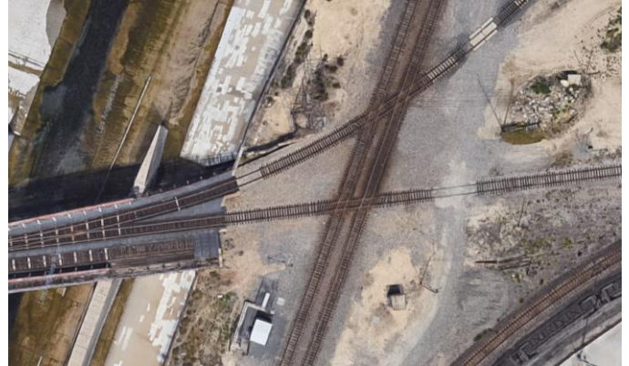
Sunset Line tracks east of Mission Junction, near crossing of Mission Junction Bridge. Satellite imagery dated 2018, courtesy of Google Maps. Note section of missing ties at right. (Track locations within the study area were unsafe and/or inaccessible for project team to photograph.)
