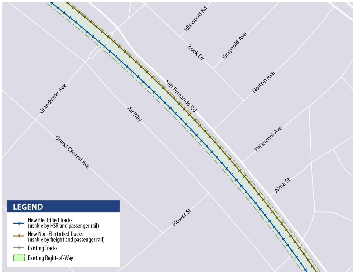
Figure 2-2 New Electrified and Non-Electrified Tracks Within Existing Right-of-Way
