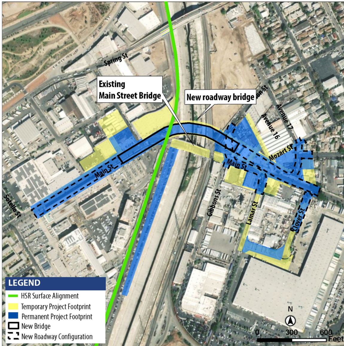
Figure 2-20 Main Street Grade Separation Footprint
