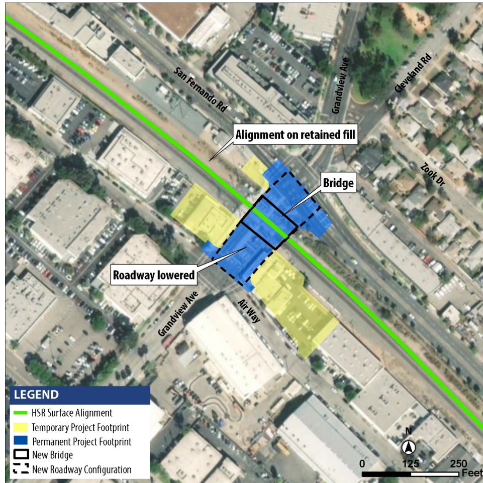
Figure 2-17 Grandview Avenue Grade Separation Footprint
