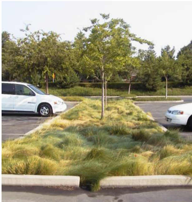
Parking lot landscaping can include water quality improvement features (LID features).
