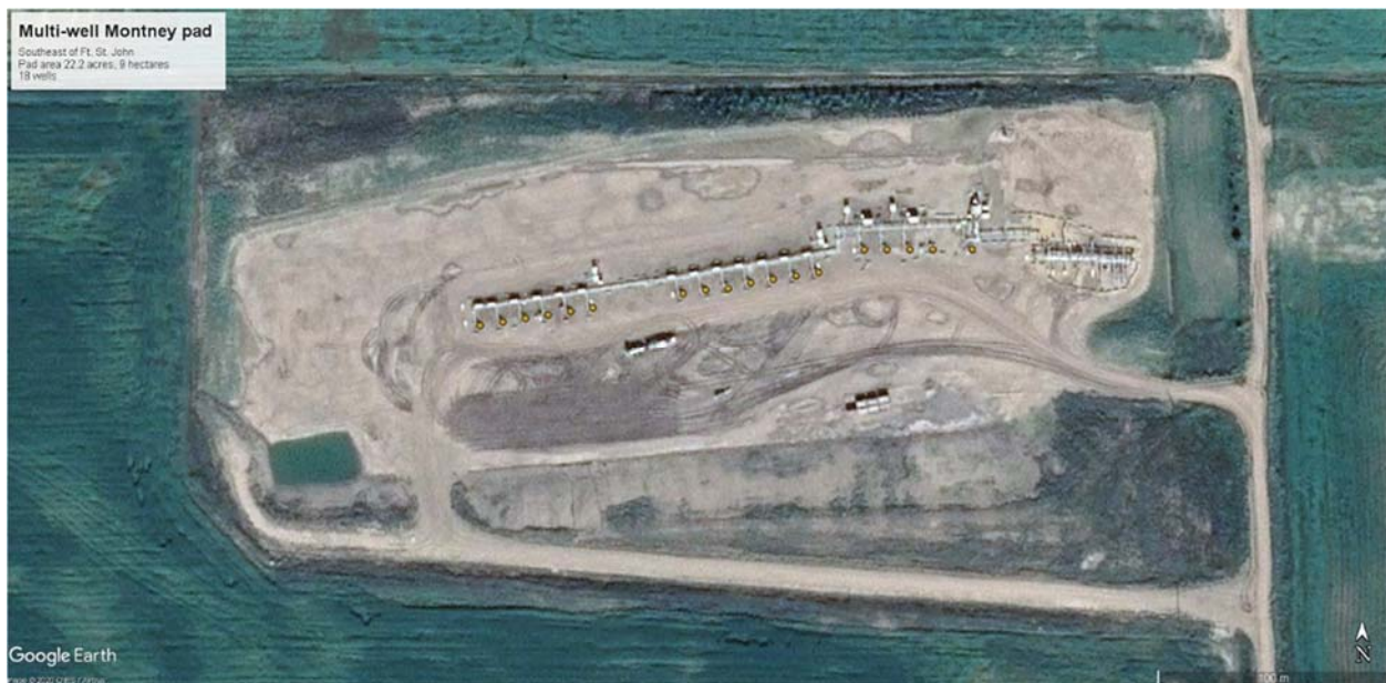
Figure 3 – Example of a multi-well pad from the Montney Formation in Canada. Eighteen wells have been drilled on this 22-acre pad. (Scale bar at lower right.)
