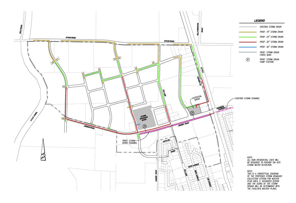
Figure 3.7: Preliminary Backbone Stormwater System Plan
