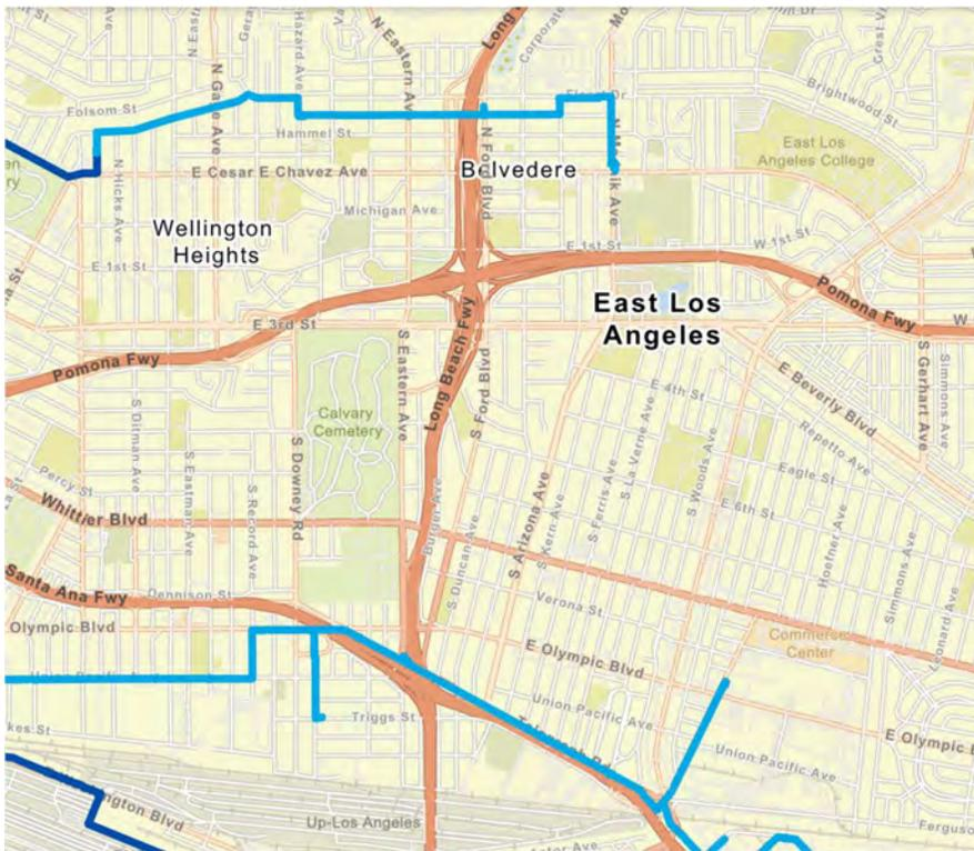
The light blue lines are high pressure distribution lines. The dark blue are transmission lines.
