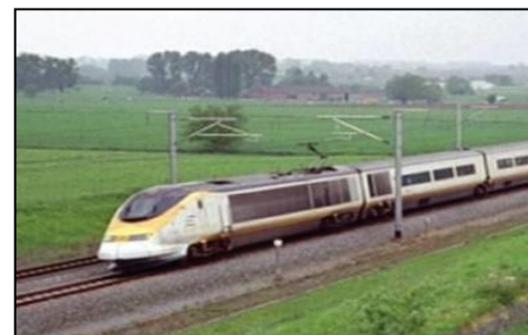
Figure 2 Example of an At-Grade Profile Showing Contact Wire System and Vertical Arms of the Pantograph Power Pickups
