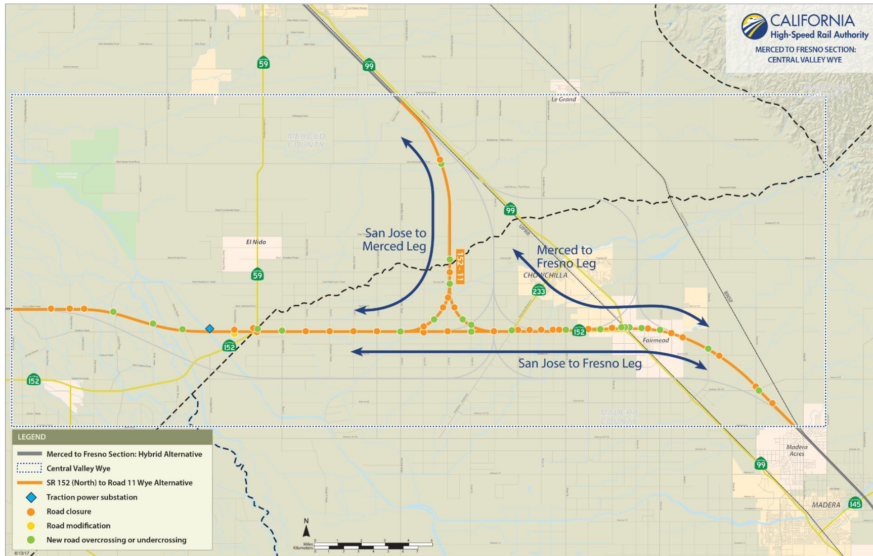
Figure 2-14 SR 152 (North) to Road 11 Wye Alternative Alignment and Key Design Features
