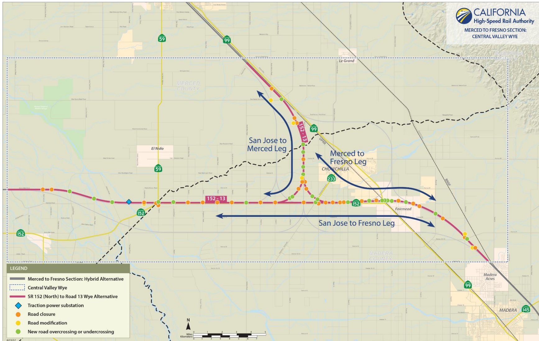
Figure 2-8 SR 152 (North) to Road 13 Wye Alternative Alignment and Key Design Features
