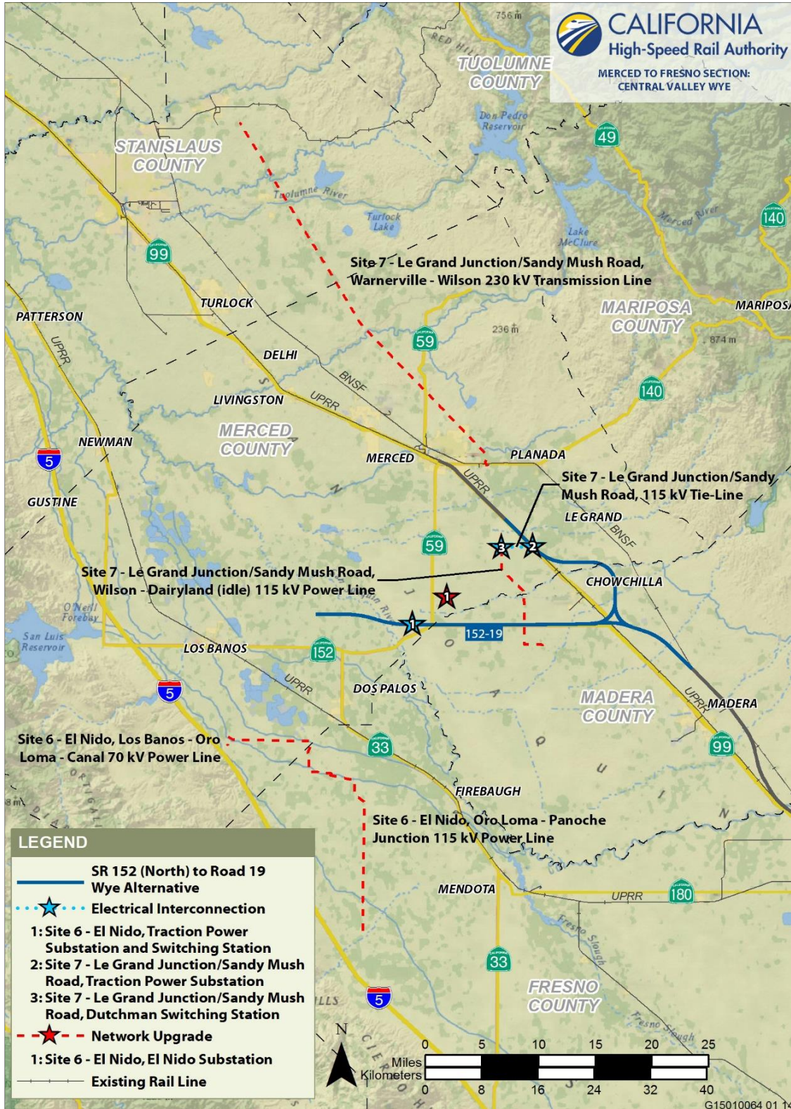
Figure 2-11 SR 152 (North) to Road 19 Wye Alternative Electrical Interconnections and Network Upgrades
