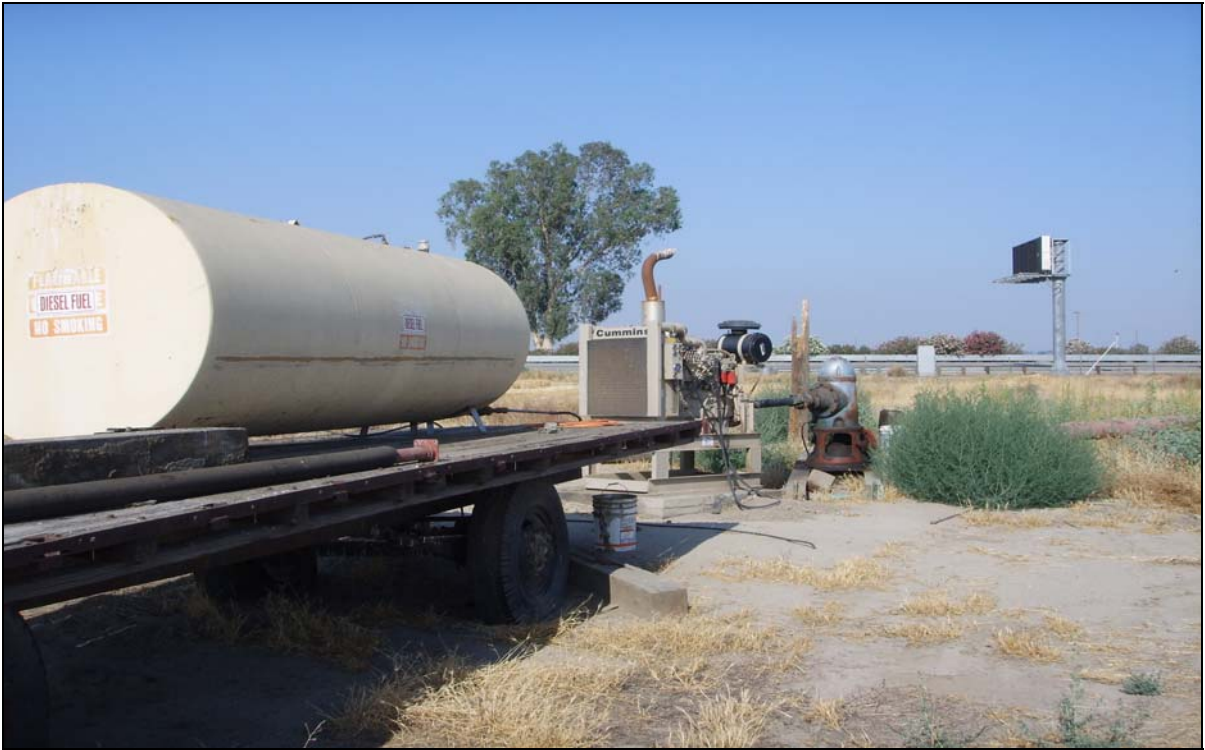
Photo 3. West-facing view of the west irrigation well with diesel engine and trailer-mounted AST.
