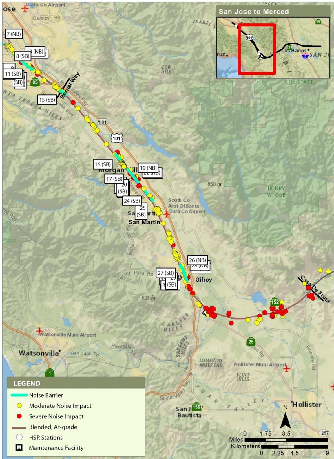
Figure 3.4-41a Proposed Noise Barriers and Residual Noise Impacts—Alternative 4 without the Tunnel Design Variant (Morgan Hill and Gilroy Subsection)
