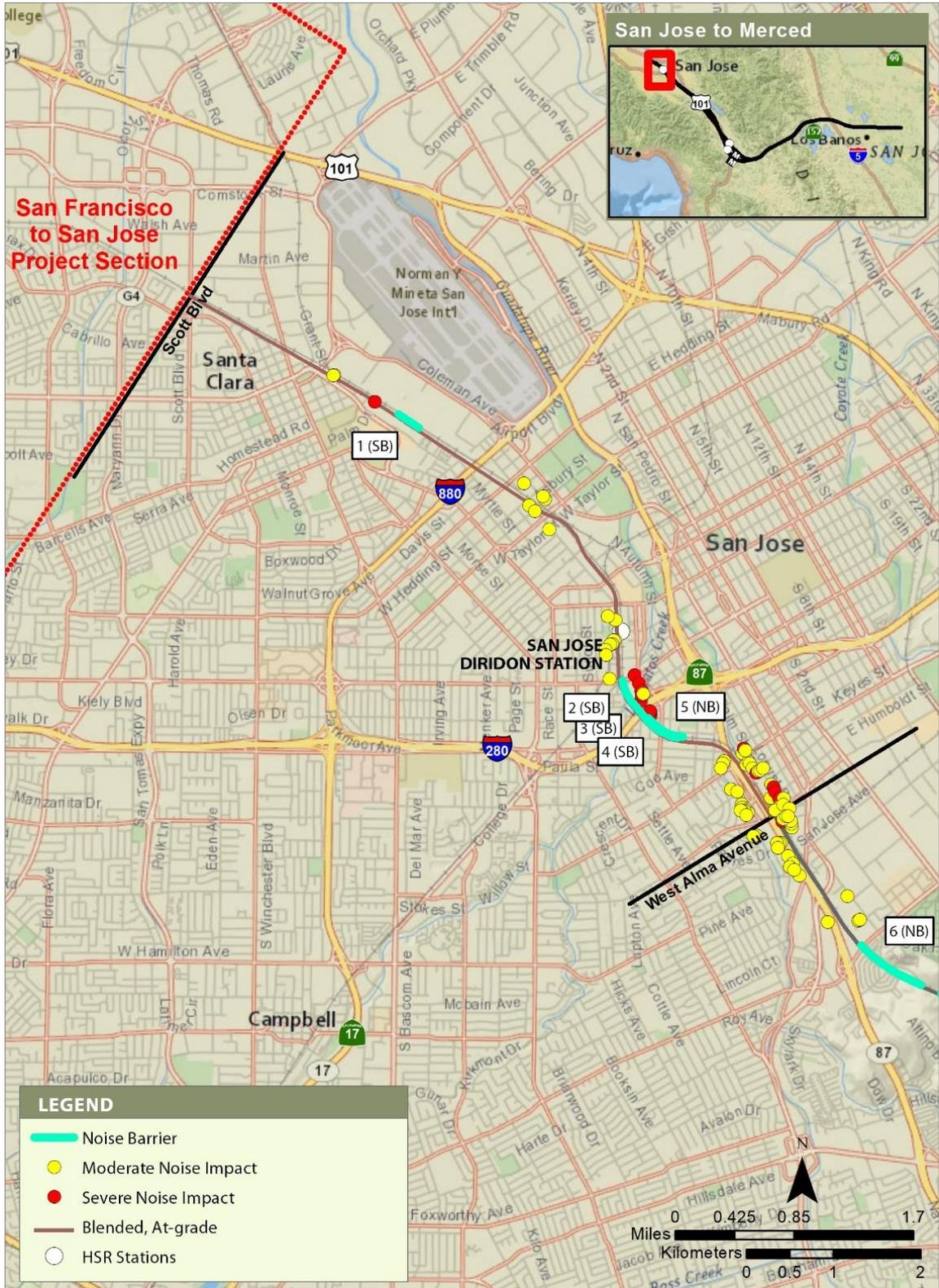
Figure 3.4-39 Proposed Noise Barriers and Residual Noise Impacts—Alternative 4 (San Jose Diridon Station Approach Subsection)
