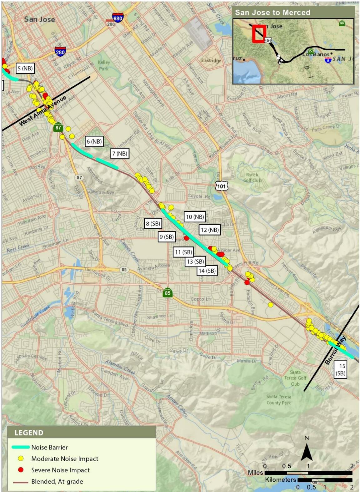
**Figure 3.4-40 Proposed Noise Barriers and Residual Noise Impacts—Alternative 4 (Monterey Corridor Subsection)**
