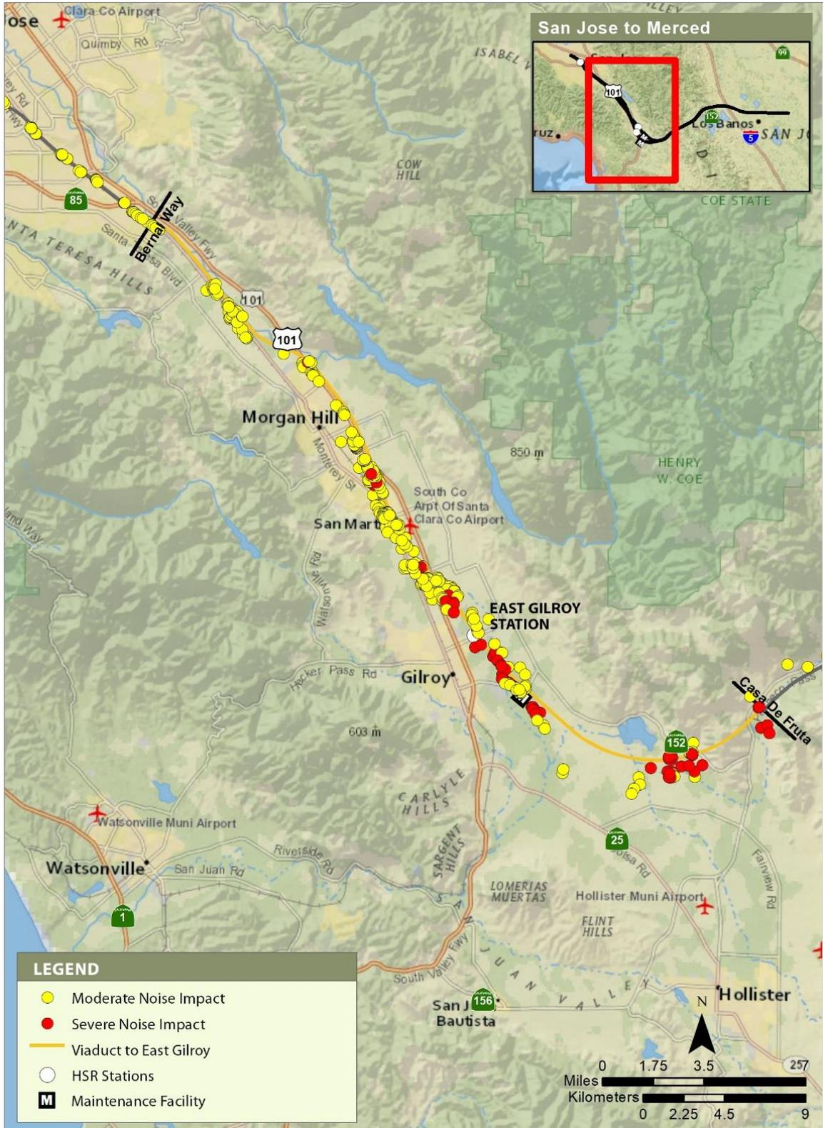
**Figure 3.4-18a 2040 Plus Project Noise Impacts—Alternative 3 without the Tunnel Design Variant (Morgan Hill and Gilroy Subsection)**
