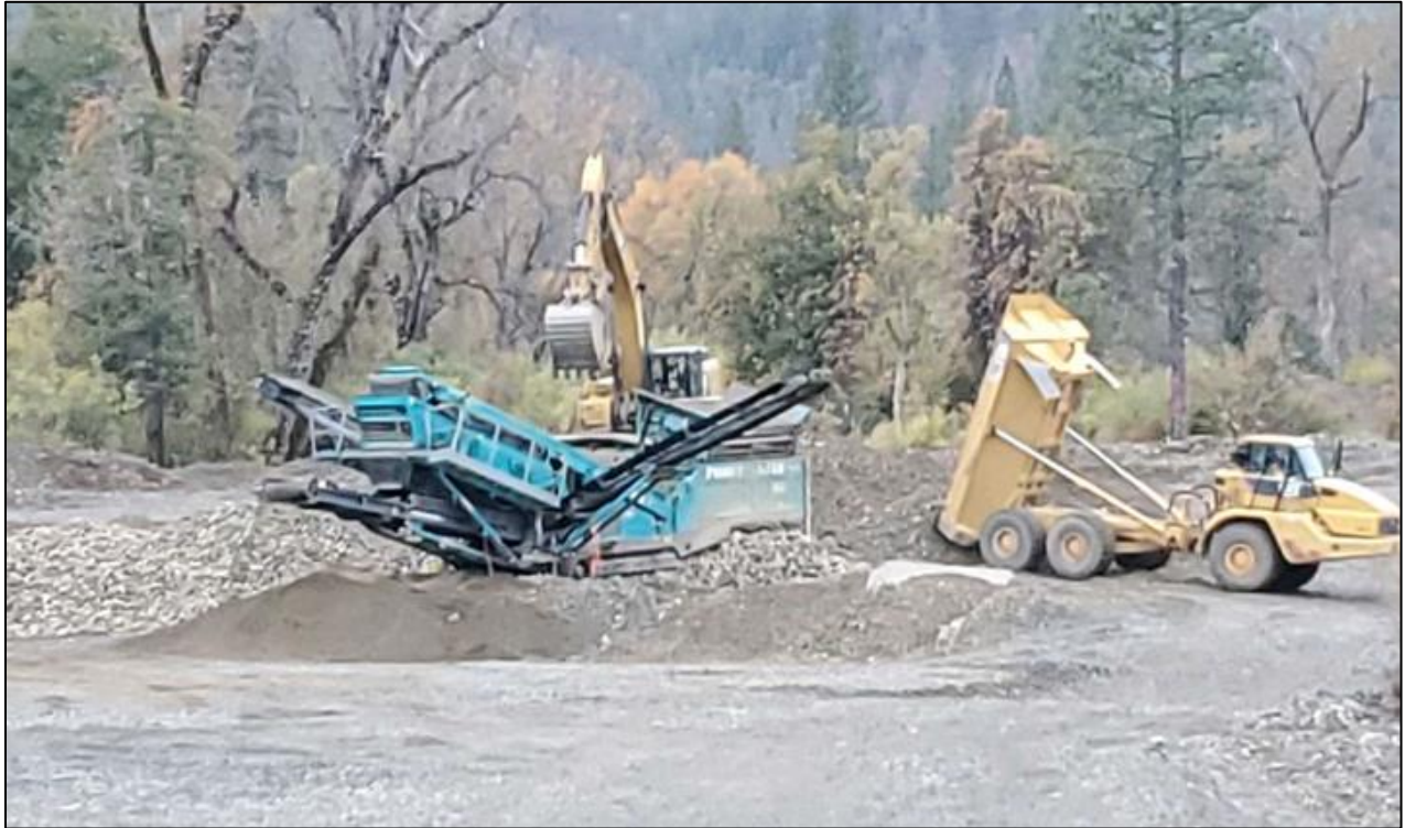
Figure 2-1. Sediment processing equipment at a restoration site, including a belt conveyor, front loader, excavator, and screening plant to sort materials by size class.
