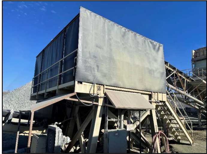
Figure 10 – Crusher GP500 after acoustic curtain installation
