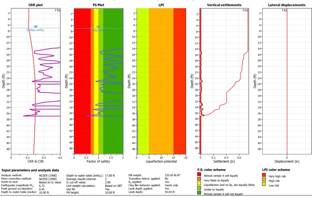
Liquefaction analysis overall plots
