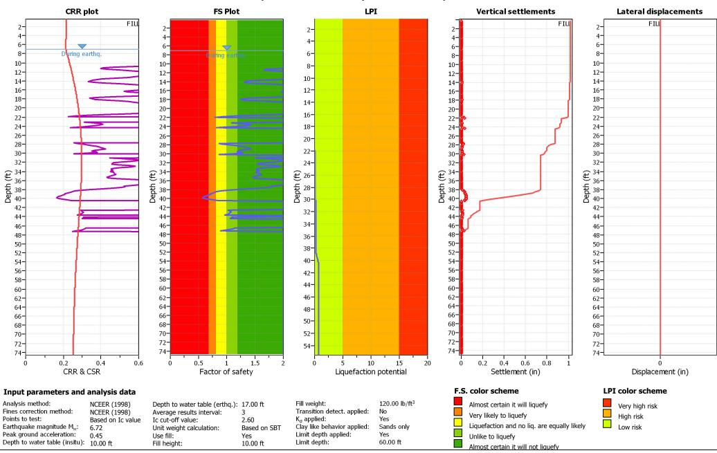
Liquefaction analysis overall plots
