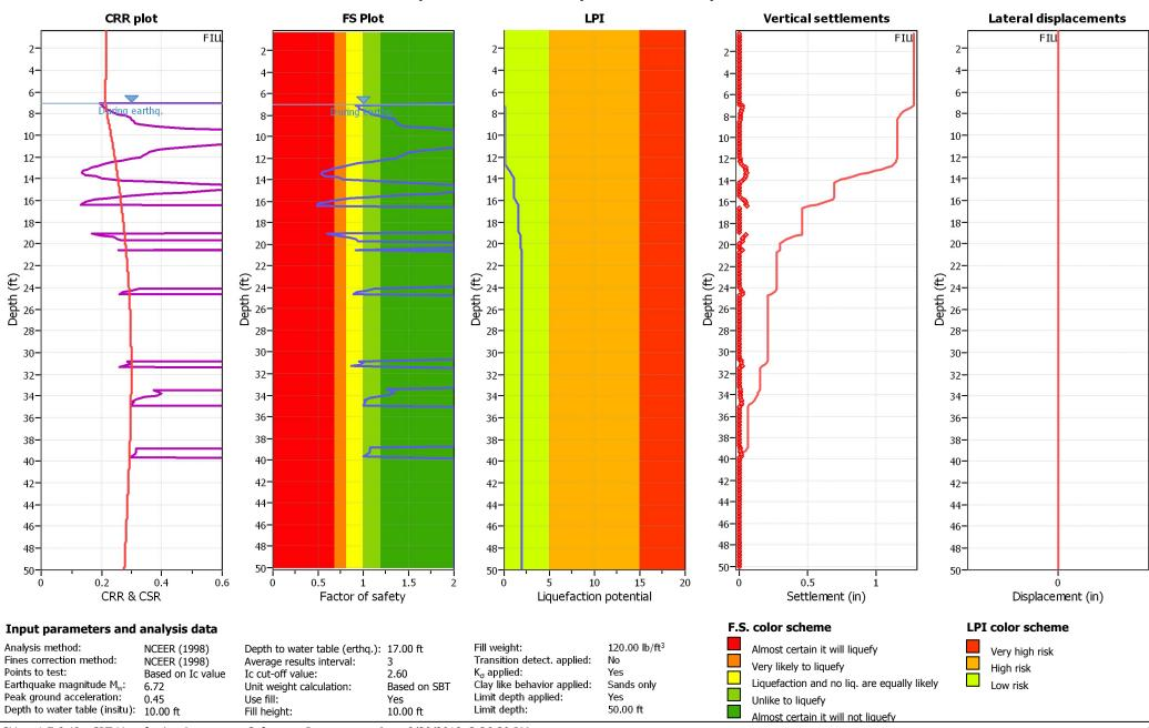
Liquefaction analysis overall plots
