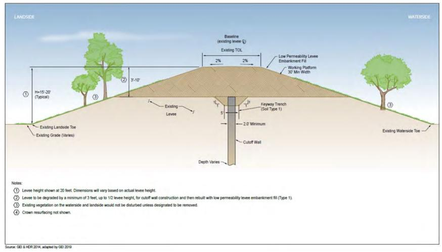
Figure 2-6 Typical Conventional Slurry Wall
