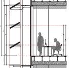
Most exposure per fin with looser spacing and rotation, but fewer total fins.
