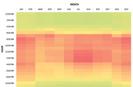
Figure 14 - Annual Marginal Greenhouse Gas Emissions Profile for Fountain Alley, without on-site PV. Relative CO2lbs/kWh electricity
