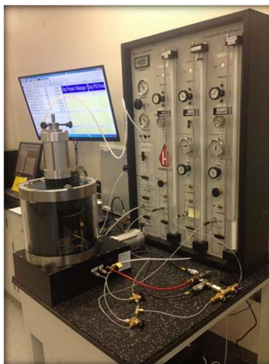
EXHIBIT 3.3.3.4-1: ENGEO CSS Apparatus
