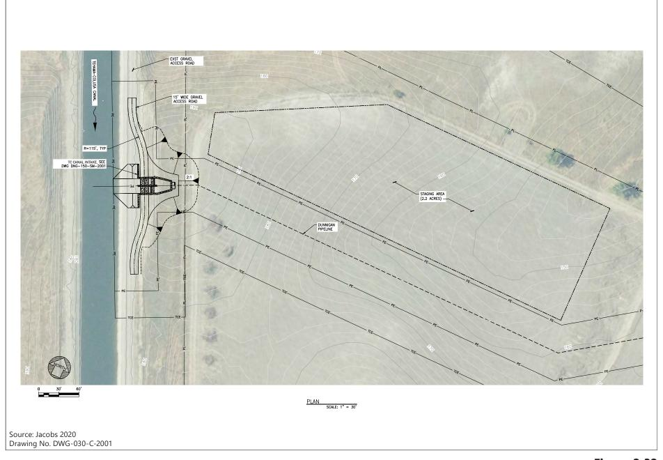
Figure 2-32 TC Canal Intake Site Plan
