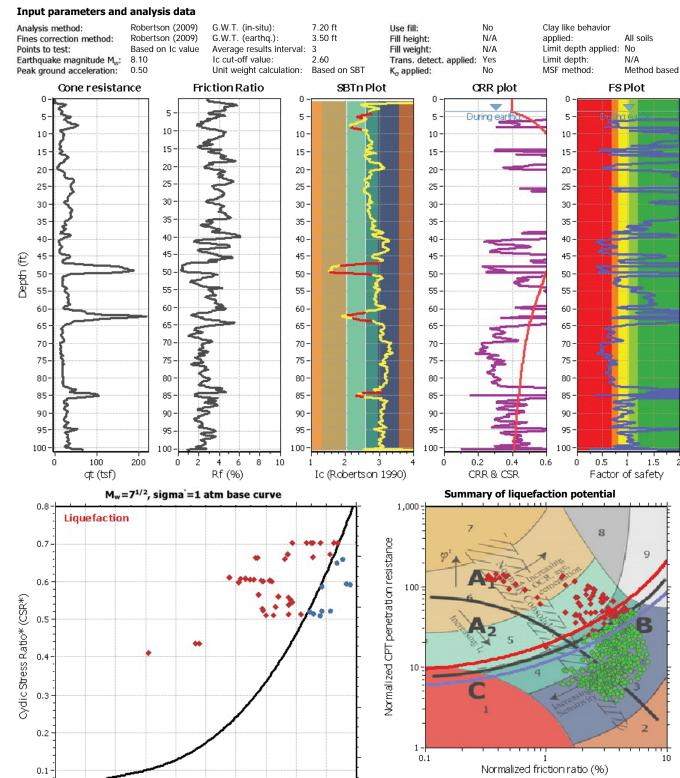
Zone  $A_{\gamma}$ : Cyclic liquefaction likely depending on size and duration of cyclic loading Zone  $A_{\gamma}$ : Cyclic liquefaction and strength loss likely depending on loading and ground geometry
